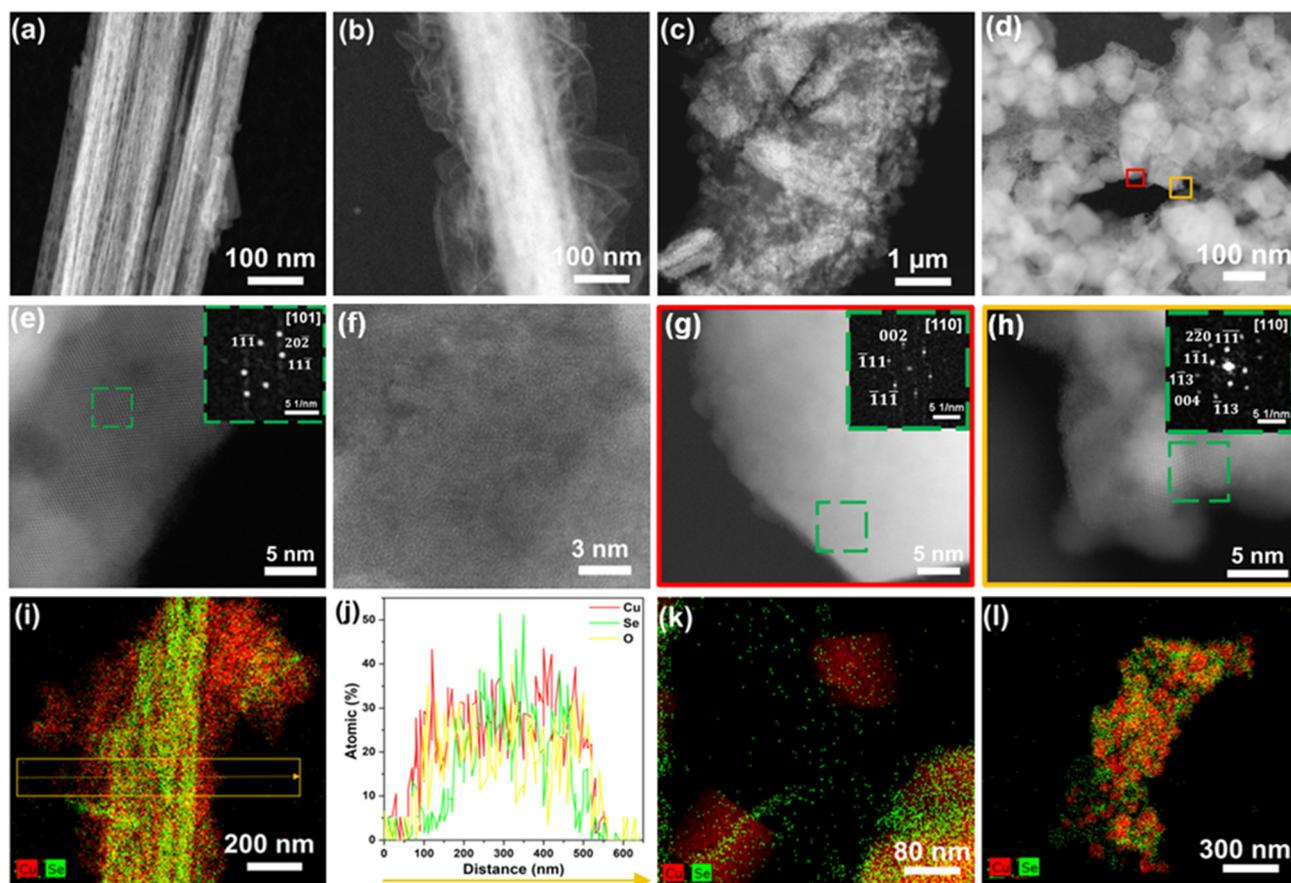
**Fig. 1** HAADF-STEM images of (a and e) AP-CuSe, (b and f) CA-CuSe, (c) EA-CuSe, (d, g and h) EA-CA-CuSe. FFT pattern insets in (e, g and h) show the zone axis and the crystalline planes of the crystal structures in the green dashed squares. EDS elemental maps of (i) CA-CuSe, (k) EA-CuSe, and (l) EA-CA-CuSe. (j) Line scan along the cross-section of the CA-CuSe nanowire in (i), which shows that Cu is preferentially present at the surface.
