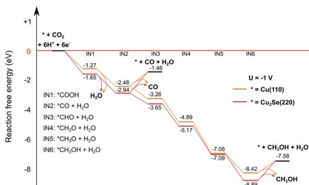
Fig. 5 Computed reaction CO<sub>2</sub>RR pathways on Cu<sub>2</sub>Se (220) and Cu (110) slab models to CO and methanol with an applied cell voltage of –1 V.
