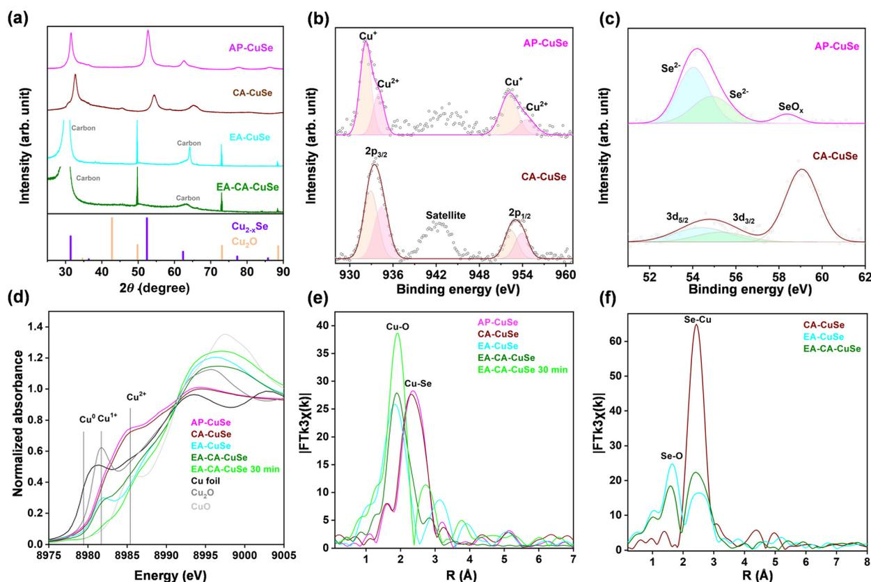
Fig. 2 (a) XRD spectra of the different  $\text{Cu}_{2-x}\text{Se}$ -based samples. XPS of AP-CuSe and CA-CuSe samples at the (b) Cu 2p and (c) Se 3d levels. (d) Cu K-edge XANES. Fourier Transforms of (e) Cu K-edge and (f) Se K-edge  $k^3$ -weighted EXAFS spectra.
