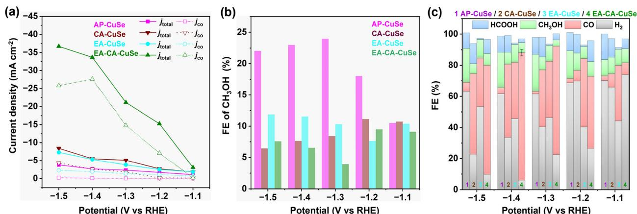
**Fig. 3** Variation with the applied potential of (a) total current density and CO partial current density, (b) FE of  $\text{CH}_3\text{OH}$  and (c) FE of all products for AP-CuSe, CA-CuSe, EA-CuSe, and EA-CA-CuSe. The error bar on  $\text{FE}_{\text{CO}}$  for EA-CA-CuSe at  $-1.4 \text{ V}_{\text{RHE}}$  is the standard deviation of triplicate measurements. For other samples and bias voltages only single measurements were performed.
