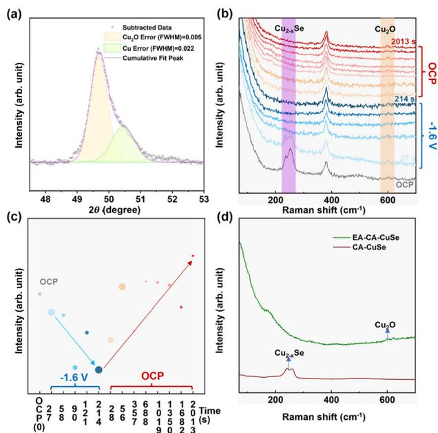
**Fig. 4** EA-CA-CuSe (a) Quasi *in situ* XRD spectra. (b) In situ Raman spectra and (c) intensity of the Raman peak at  $600\text{ cm}^{-1}$  in (b) as a function of the time during which  $-1.6\text{ V}_{\text{RHE}}$  is applied (blue symbols) or at OCP (red symbols). The size of the symbol represents the error bar. (d) Ex situ Raman spectra of CA-CuSe and EA-CA-CuSe.
