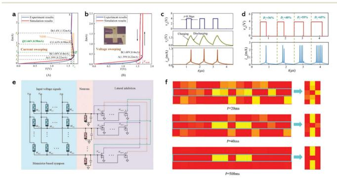
Fig. 18 (a) Current sweep I-V plot. (b) Voltage sweep I-V plot. (c) Neuromorphic behaviors under the 0.36  $\mu$ s voltage pulse. (d) Neuromorphic behaviors under different input pulse widths. (e) Circuit construction of memristor neuron networks. (f) Change in the resistance value of the synaptic array of the memristor after the input of "H" (which constitutes the input vector using high and low levels of voltage).<sup>230</sup>
