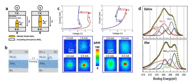
Fig. 6 (a) Metallic rutile NbO<sub>2</sub> nucleation process during electroforming.  $^{152}$  (b) Schematics of the electroforming mechanisms in the NbO<sub>x</sub> device.  $^{153}$  (c) Electroforming characteristic and *in situ* thermos reflectance mapping of devices with areas measuring 5  $\times$  5  $\mu$ m<sup>2</sup> and 10  $\times$  10  $\mu$ m<sup>2</sup>.  $^{154}$  (d) XPS spectra before and after electroforming.  $^{155}$
