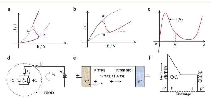
Fig. 1 Current-voltage dependence curves of (a) S-shaped and (b) N-shaped NDR devices. 9 The blue dashed lines show the field-induced transition that occurs between states a and b. 13 (c) I-V characteristics of the Esaki diode. (d) A simple equivalent circuit of an Esaki diode connected to a battery. 14 (e) Structure of IMPATT. (f) Fixed charge and field distributions in various regions. 15
