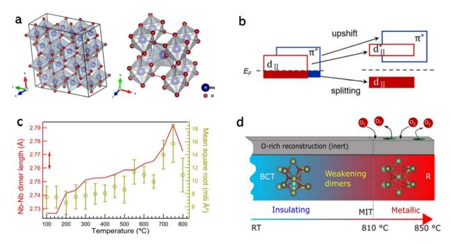
Fig. 7 (a) Body-centered tetragonal phase and rutile phase of niobium oxide.  $^{163}$  (b)  $d_{\parallel}$  energy band split during MIT.  $^{126}$  (c) Nb-Nb dimer length variation with temperature, which is characterized by temperature-dependent extended X-ray absorption fine structure spectroscopy (T-EXAFS). (d) Schematic representation of the insulator-metal transition of niobium oxide.  $^{164}$
