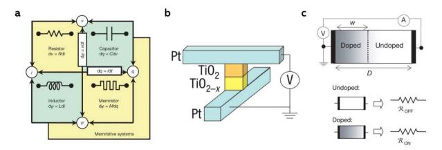
Fig. 3 (a) Relationship between basic passive circuit elements and basic circuit variables. (b) Fabric of Pt/TiO<sub>2</sub>/Pt memristor. (c) Conception of the resistive switching principle. 108
