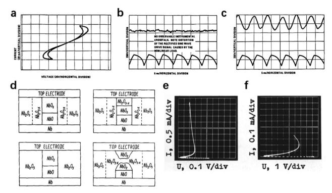
Fig. 5 (a) I-V characteristic of the NbO<sub>2</sub> device. (b) Temporal modulation response of a device in the absence of light. (c) Temporal modulation of the device under high illumination. <sup>143</sup> (d) Phase diagram of different phase distributions of a-Nb<sub>2</sub>O<sub>5</sub> film. (e) I-V characteristics of current channels in the high conductivity state. (f) I-V characteristics of current channels in a low conductivity state.
