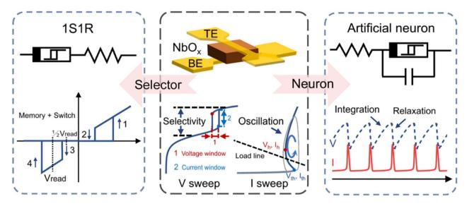
Fig. 4 Typical structure of a niobium oxide device: top electrode, niobium oxide functional layer, and bottom electrode. Threshold switching imagery under voltage scanning, and negative differential resistance effects under current scanning. Niobium oxide memristor is used as a selector or neuron by combining it with an electronic component, and the electrical characterization of both of them.<sup>126</sup>
