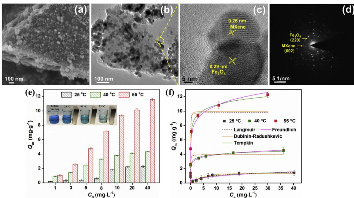
**Fig. 13** (a) SEM, (b) TEM, (c) HRTEM, (d) SAED pattern of 2D-MX@Fe<sub>3</sub>O<sub>4</sub> nanocomposites. (e) The removal capacity of MB over 2D-MX@Fe<sub>3</sub>O<sub>4</sub> at 25, 40 and 55 °C. (f) Adsorption isotherms of 2D-MX@Fe<sub>3</sub>O<sub>4</sub> for MB removal. Reproduced with permission from ref. 145. Copyright 2019, Elsevier.
