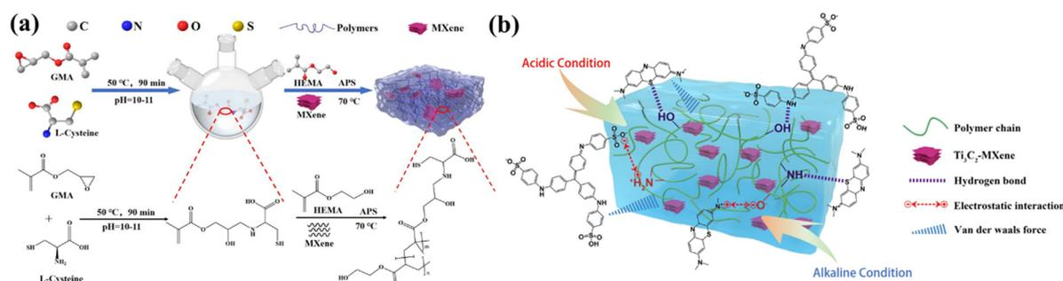
Fig. 11 (a) Schematic preparation of PHGC/MXene hydrogel; (b) adsorption mechanism diagram of PHGC/MXene for AB93 or MB. Reproduced with permission from ref. 135. Copyright 2019, Elsevier.
