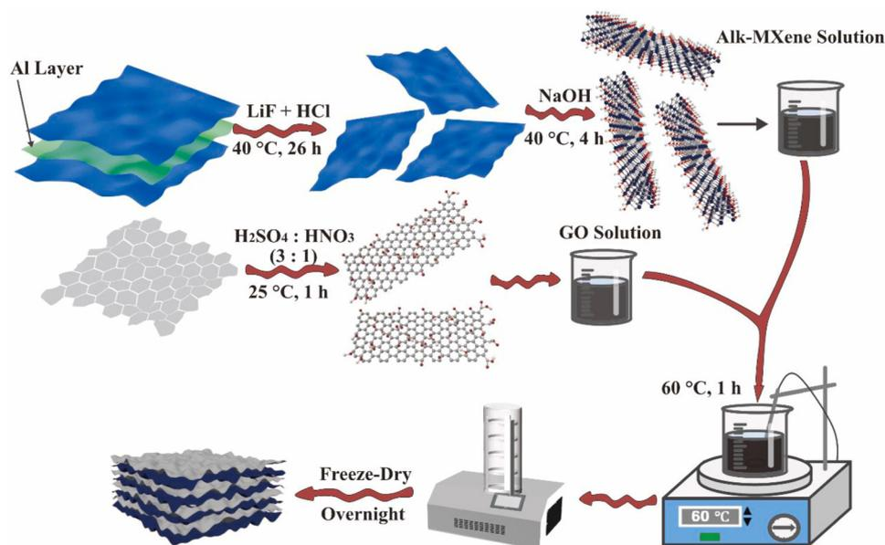
Fig. 10 Diagram for the preparation of AMXGO. Reproduced with permission from ref. 147. Copyright 2024, Elsevier.
