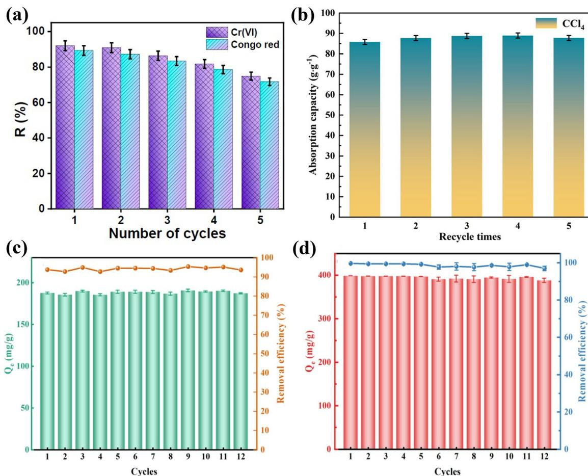
**Fig. 17** Reusability tests for (a)  $\text{Ti}_3\text{C}_2\text{T}_x/\text{NiFeMn-LDH@Gel}$  against Cr(vi) and CR. Reproduced with permission from ref. 146. Copyright 2024, Elsevier. (b)  $\text{TiVCT}_x/\text{Gas}$  against  $\text{CCl}_4$ . Reproduced with permission from ref. 156. Copyright 2024, American Chemical Society. Studies on the regeneration of (c) AB93 and (d) MB by PHGC/MXene. Reproduced with permission from ref. 135. Copyright 2024, Elsevier.
