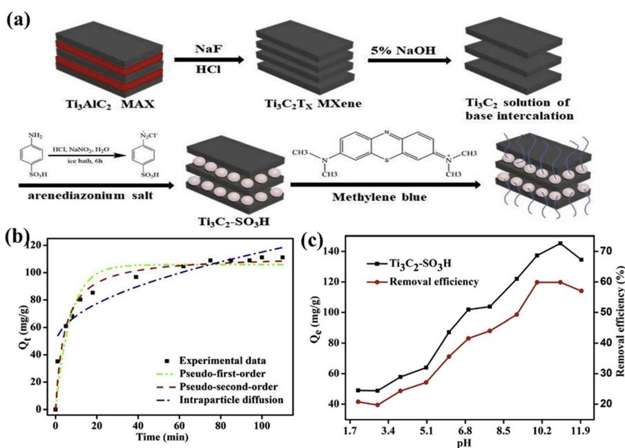
Fig. 7 (a) Schematic diagram for the preparation of  $\text{Ti}_3\text{C}_2\text{-SO}_3\text{H}$  for MB removal. (b) The kinetic curves of  $\text{Ti}_3\text{C}_2\text{-SO}_3\text{H}$  adsorption MB. (c) Effect of pH on the adsorption of MB onto  $\text{Ti}_3\text{C}_2\text{-SO}_3\text{H}$ . Reproduced with permission from ref. 133. Copyright 2019, Elsevier.
