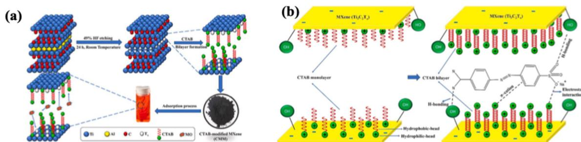
**Fig. 8** (a) Illustration of the intercalation of CTAB in MXene (CMM) for the adsorption of MO; (b) CTAB monolayer and bilayer formation on MXene ( $\text{Ti}_3\text{C}_2\text{T}_x$ ) sheets and adsorption mechanisms of MO by MXene sheets. Reproduced with permission from ref. 136. Copyright 2024, Elsevier.
