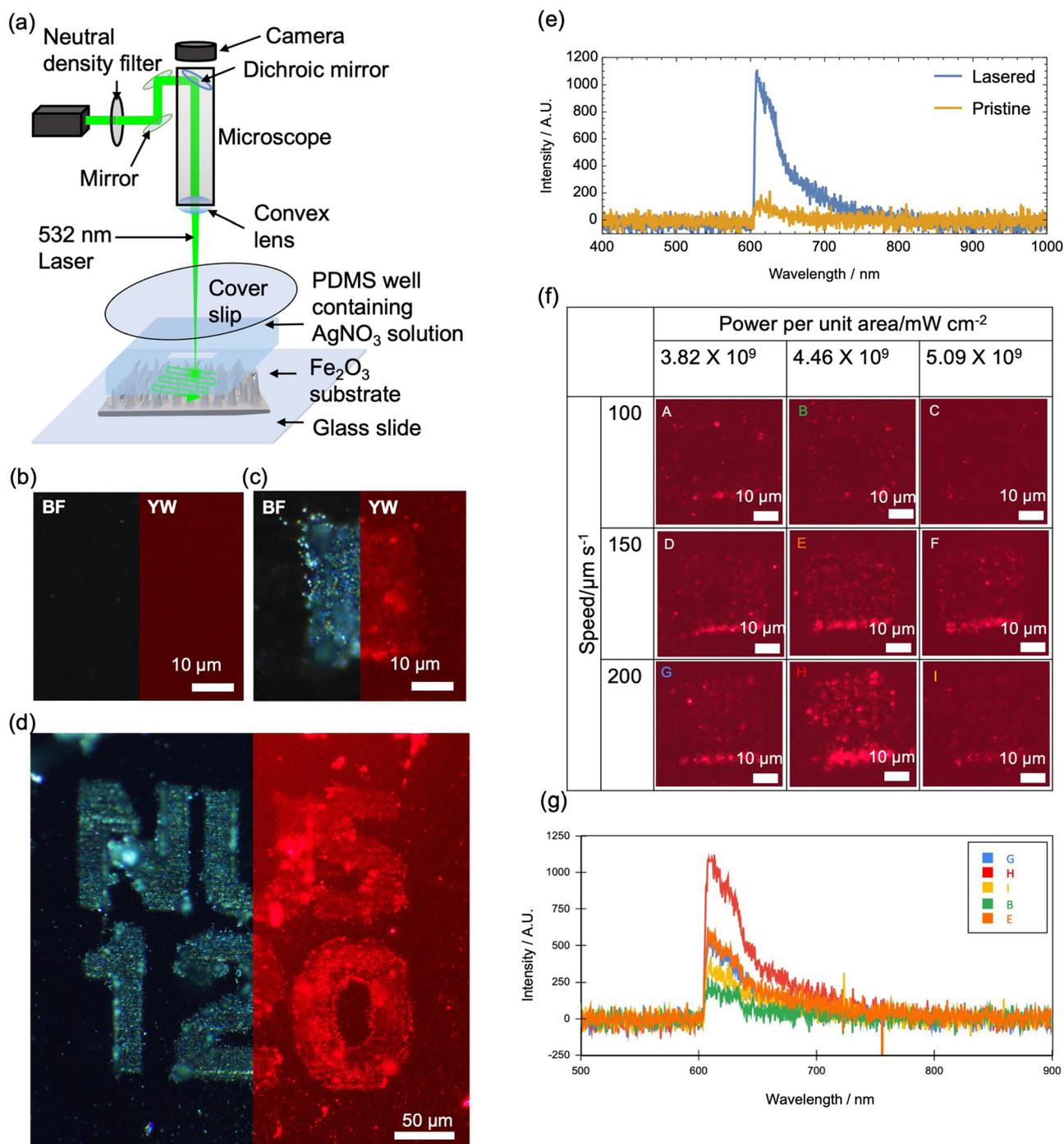
**Fig. 2** (a) Schematic of the focused laser beam set-up. (b) Pristine sample and (c) lasered micro square under bright field (left) and yellow excitation (right). (d) Micro pattern of words "NUS 120" observed under bright field (left) and yellow excitation (right). (e) FM spectra of the pristine and lasered samples under yellow excitation. (f) FM images of lasered squares with various lasering parameters and (g) the corresponding fluorescence spectra from (f).
