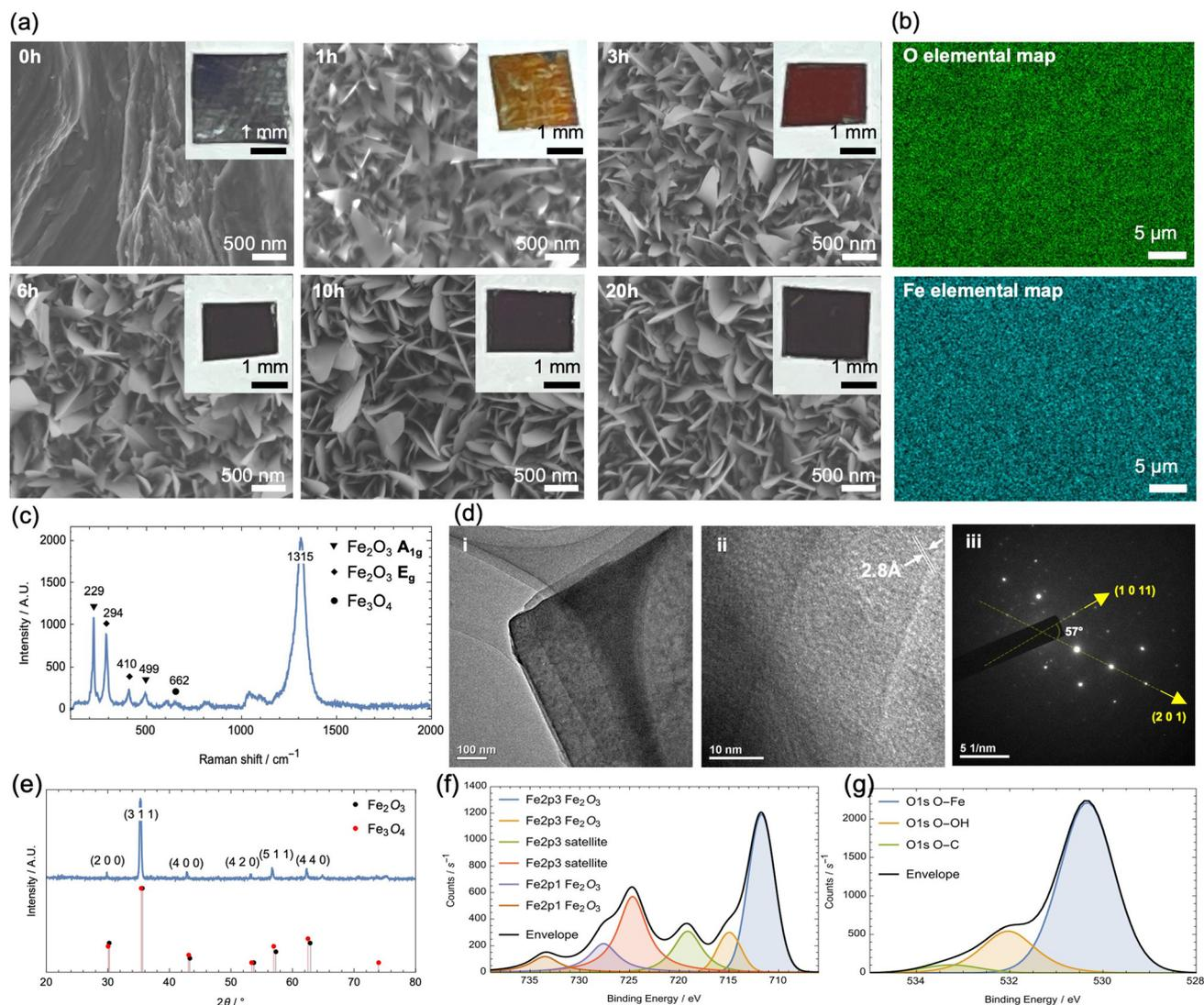
**Fig. 1** (a) SEM images of the iron oxide nanoflakes formed after 0, 1, 3, 6, 10 and 20 hours of growth, with the corresponding optical images shown in the inset. (b) EDX elemental map of O and Fe elements, (c) Raman spectrum, (d) (i) TEM image, (ii) high-resolution TEM (HRTEM) image, (iii) SAED pattern, (e) XRD results and (f and g) XPS spectra showing the (f) Fe 2p and (g) O 1s scans of the iron oxide nanoflakes after 20 hours of growth.
