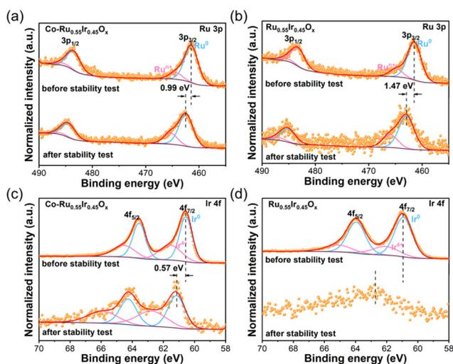
**Fig. 3** XPS spectra of Ru 3p of (a) Co-Ru<sub>0.55</sub>Ir<sub>0.45</sub>O<sub>x</sub> and (b) Ru<sub>0.55</sub>Ir<sub>0.45</sub>O<sub>x</sub> before and after the HER stability test. XPS spectra of Ir 4f of (c) Co-Ru<sub>0.55</sub>Ir<sub>0.45</sub>O<sub>x</sub> and (d) Ru<sub>0.55</sub>Ir<sub>0.45</sub>O<sub>x</sub> before and after the HER stability test.
