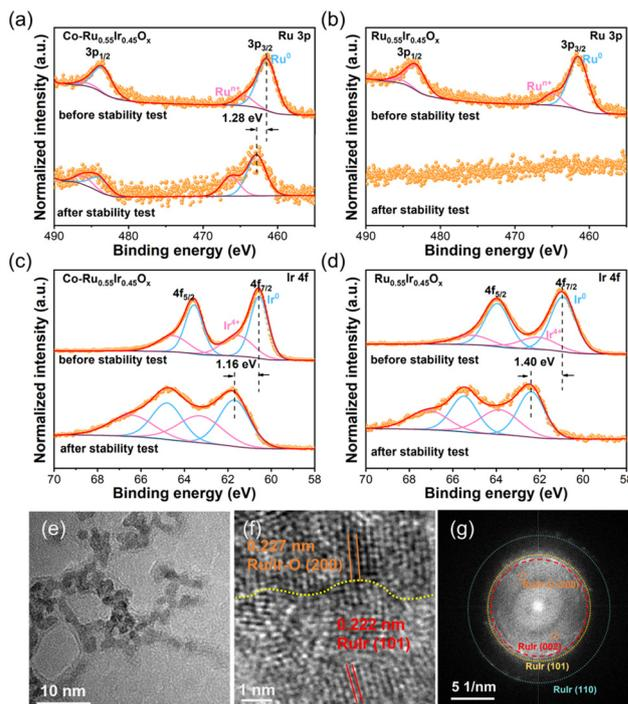
**Fig. 5** XPS spectra of Ru 3p of (a) Co-Ru<sub>0.55</sub>Ir<sub>0.45</sub>O<sub>x</sub> and (b) Ru<sub>0.55</sub>Ir<sub>0.45</sub>O<sub>x</sub> before and after the OER stability test. XPS spectra of Ir 4f of (c) Co-Ru<sub>0.55</sub>Ir<sub>0.45</sub>O<sub>x</sub> and (d) Ru<sub>0.55</sub>Ir<sub>0.45</sub>O<sub>x</sub> before and after the OER stability test. TEM image (e), HR-TEM image (f) and relevant FFT (g) of Co-Ru<sub>0.55</sub>Ir<sub>0.45</sub>O<sub>x</sub> after the OER stability test.
