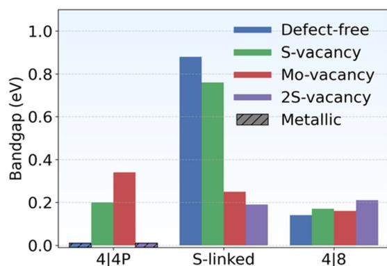
**Fig. 3** Bandgaps of representative mirror twin grain boundaries (4|4P, S-linked, and 4|8) under different defect conditions—defect-free, single sulphur vacancy, single molybdenum vacancy, and double sulphur vacancy—plotted from left to right for each GB.
