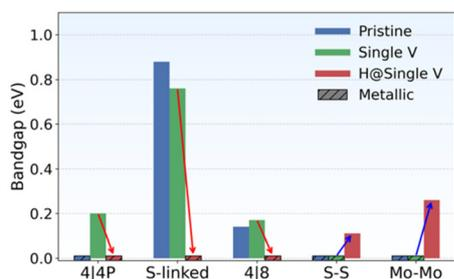
**Fig. 8** Bandgaps of various grain boundaries under three structural conditions—defect-free, single-defective and hydrogenated—plotted from left to right for each GB. Red arrows show the restoration of metallicity by hydrogenation, while the blue arrows show bandgap opening by hydrogenation.
