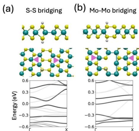
**Fig. 7** Fully relaxed atomic configuration of GBs with hydrogenation at the position of point defects. Two metallic types of GBs are investigated: (a) S–S bridging GB with single sulphur vacancies and (b) Mo–Mo bridging GB with single Mo vacancies. The Fermi levels are aligned to 0 in all band structure plots. The side view and top view are provided for clear observation of the positions of the hydrogen atoms.
