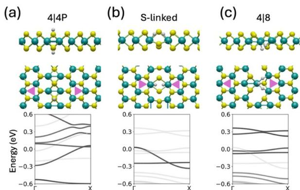
**Fig. 6** Fully relaxed atomic configuration of GBs with hydrogenation at the position of point defects. Three semiconducting types of GBs are investigated: (a) 4|4P, (b) S-linked GB and (c) 4|8 with single sulphur vacancies. The Fermi levels are aligned to 0 in all band structure plots. The side view and top view are provided for clear observation of the positions of the hydrogen atoms.
