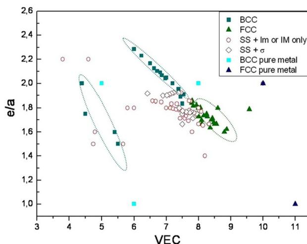
Fig. 3 VEC and itinerant electron ( $e/a$ ) plot of various multielement systems. Highlighted correlation of lower VEC and high  $e/a$  predicts BCC phase formation. Reproduced from ref. 52 Copyright (2014), with permission from Elsevier.
