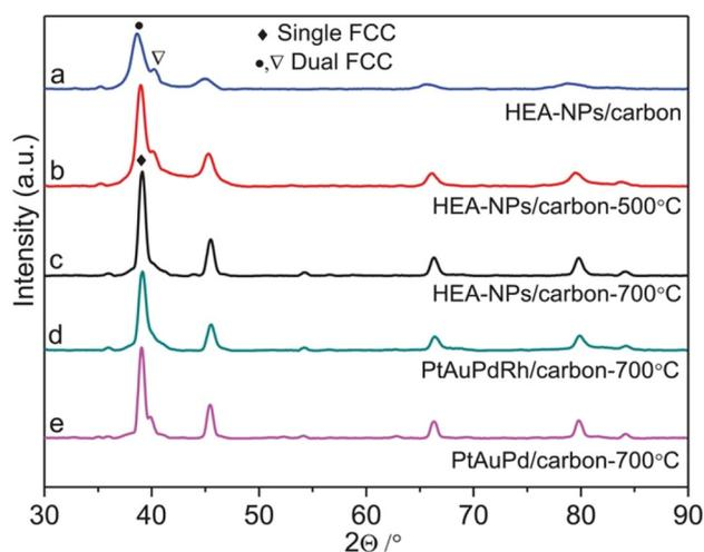
**Fig. 10** XRD patterns of synthesized HEA-NPs/carbon prepared via the ultrasonication-assisted wet chemistry method: (a) before calcination under  $N_2$ , (b) after calcination under  $N_2$  at 500 °C for 2 hours, and (c) at 700 °C for 2 hours. Additionally, XRD patterns of (d) PtAuPdRh/carbon and (e) PtAuPd/carbon, both synthesized using the same method and calcined under  $N_2$  at 700 °C for 2 hours. Reproduced from ref. 78 Copyright (2022), with permission from Wiley.
