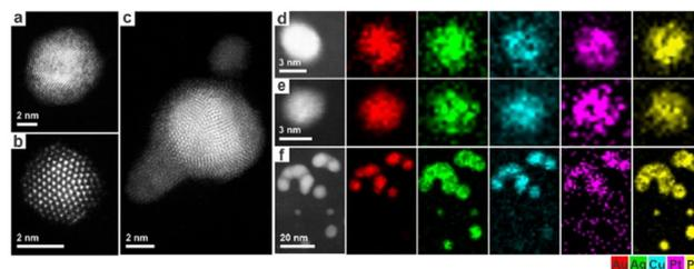
**Fig. 17** AuAgCuPtPd HEA NPs synthesized with different metal:ligand ratios: (a and d) 1:1, (b and e) 2.5:1, and (c and f) 5:1. (a–c) HAADF-STEM images of HEA NPs, with corresponding EDS elemental maps shown in (d–f). Reproduced from ref. 124 Copyright (2023), with permission from RSC publishing.
