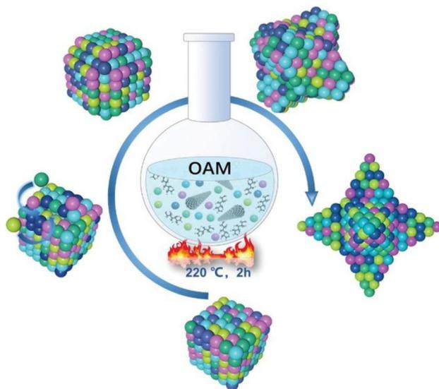
**Scheme 3** Schematic of the synthesis of convex cube-shaped Pt<sub>34</sub>Fe<sub>5</sub>Ni<sub>20</sub>Cu<sub>31</sub>Mo<sub>9</sub> HEA on CNT-support. Reproduced from ref. 74 Copyright (2022), with permission from Wiley.
