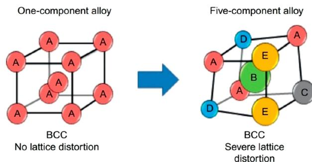
**Scheme 1** Example of BCC lattice distortion present in high entropy alloys compared to traditional alloys. Reproduced under terms of the CC-BY license.<sup>22</sup> Copyright (2019), W. Dong, Z. Zhou, M. Zhang, Y. Ma, P. Yu, P. K. Liaw, G. Li, published by MDPI.
