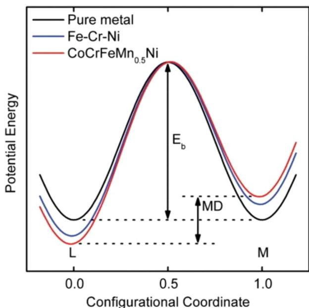
**Fig. 2** A potential energy plot illustrating the energy variation during the migration of a Ni atom. In pure metals, the mean difference (MD) in potential energy after each migration is zero, whereas HEAs exhibit the largest energy fluctuation. Reproduced from ref. 23 Copyright (2013), with permission from Elsevier.
