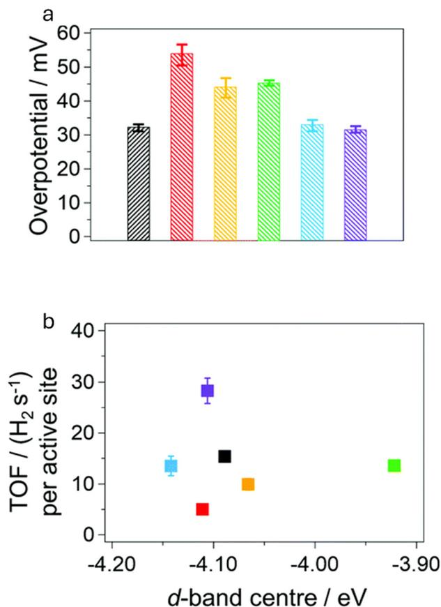
Fig. 7 (a) Overpotential of various HEA composition at  $50 \text{ mA cm}^{-2}$ . (b) Turn over frequency compared with d-band centre. Reproduced from ref. 67 Copyright (2022), with permission from RSC publishing.
