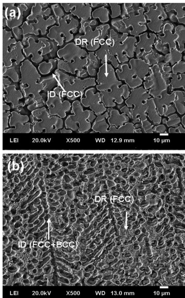
Fig. 5 Scanning electron microscope (SEM) images of  $CuCrFeNiMn$  alloy systems: (a)  $CuCr_2Fe_2Ni_2Mn_2$ , (b)  $Cu_2CrFe_2NiMn_2$ . Reproduced from ref. 66 Copyright (2011), with permission from Wiley.
