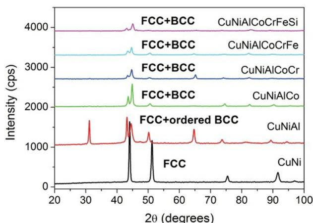
**Fig. 1** The XRD patterns of a series of alloys starting from the standard low entropy to mid entropy and eventually to high entropy alloy *via* sequential elemental addition. All the alloys have one or two major phases that have simple structures. Reproduced under terms of the CC-BY license.<sup>8</sup> Copyright (2014), M.-H. Tsai, J.-W. Yeh, published by Taylor & Francis.
