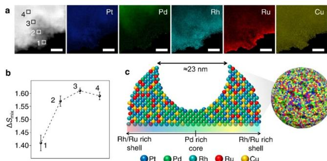
**Fig. 14** (a) PtPdRhRuCu MMN edge pore HAADF-STEM image and Energy-Dispersive X-ray Spectroscopy (EDS) maps (scale bar: 10 nm). (b)  $\Delta S_{\text{mix}}$  value at the selected area found in (a) (1–4). (c) Elemental distribution of mesopore in PtPdRhRuCu MMN. Reproduced under terms of the CC-BY license.<sup>75</sup> Copyright (2023), Y. Kang, O. Cretu, J. Kikkawa, K. Kimoto, H. Nara, A. S. Nugraha, H. Kawamoto, M. Eguchi, T. Liao, Z. Sun, T. Asahi, Y. Yamauchi, published by Springer Nature.
