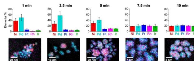
**Fig. 19** EDS maps of NiPdPtRhIr HEA NP formation at various time intervals (1, 2.5, 5, 7.5, and 10 minutes), accompanied by bar charts illustrating the corresponding elemental composition changes. Reproduced from ref. 125 Copyright (2023), with permission from American chemical society.
