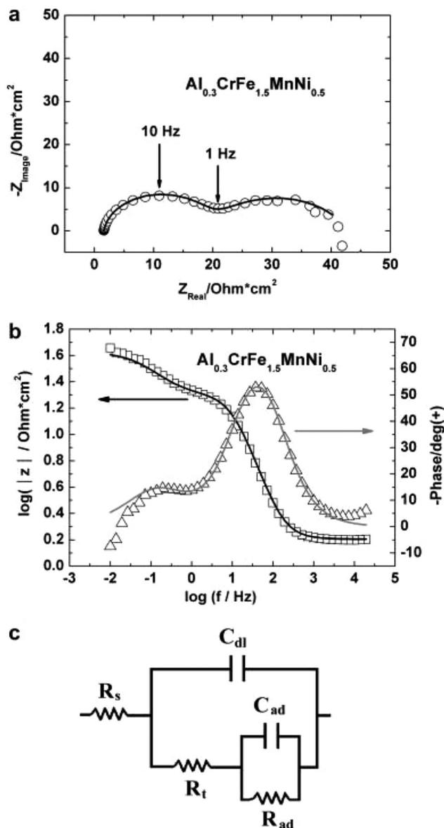
**Fig. 4** EIS results for  $\text{CrFe}_{1.5}\text{MnNi}_{0.5}$  alloy in 0.5 M  $\text{H}_2\text{SO}_4$  solution. Nyquist (a) and Bode (b) plots along with (c) equivalent electrical circuit. Scattered points represent raw experimental data points, and solid lines represent model fit. Reproduced from ref. 65 Copyright (2008), with permission from Elsevier.
