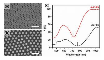
Fig. 2 SEM images of (a) AuFoN and (b) AuFoEN substrates, and (c) their corresponding reflectance spectra. Scale-bar in (a) and (b) is 1 µm.
