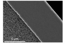
Fig. 4 Scanning electron microscopy images of the shadow mask with a 7 μm wide, 1 mm long Si bridge at different magnifications (enlargements of the dashed boxes are shown on the right). The image on the right reveals the steep sidewalls with a characteristic scalloped profile, arising from the alternating passivation and etching cycles during the Bosch DRIE process.
