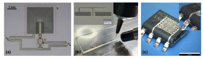
Fig. 5 Demonstrator applications for droplet-based printed electronics. (a) Low-pass filter with capacitor and inductor elements. (b) Passive components for high frequency electronics, including transmission lines and radial stubs. (c) Humidity sensor printed directly onto a packaged integrated circuit. Graphics adapted with permission from ref. 201 and 208 (CC BY), and ref. 230 (CC BY), respectively.
