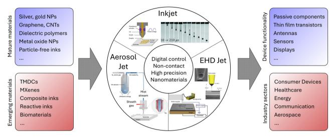
Fig. 1 Overview of droplet-based printing technologies for functional devices. Inkjet, aerosol jet, and EHD jet printing are the focus of this report, given their high-level similarities in materials requirements and process integration characteristics. Graphics adapted with permission from ref. 14 and 15 (CC BY), ref. 16 and 179 (Copyright 2009 American Chemical Society).
