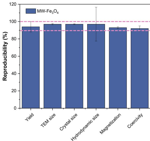
Fig. 2 Reproducibility of MW-Fe<sub>3</sub>O<sub>4</sub> (Z = 8).
