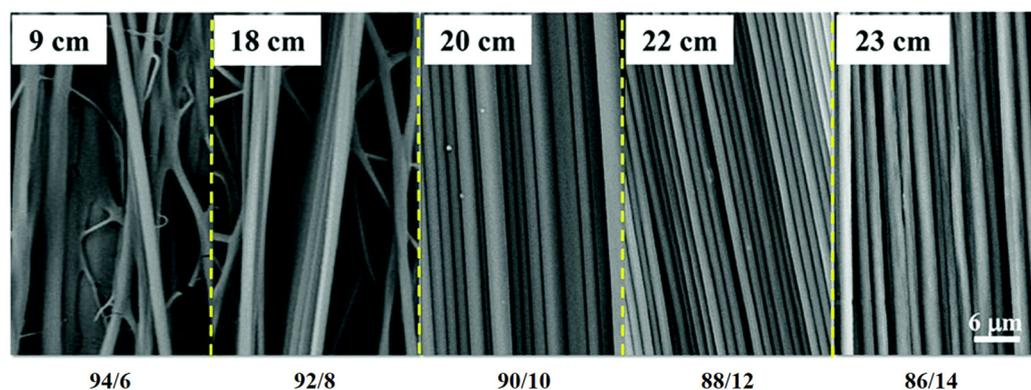
**Fig. 5** Morphologies of well-aligned silk fibroin/PEO fibers with different polymer contents collected at different stable jet lengths using SJES. The operating voltage, pumping rate, and rotating electrode speed are 8.5 kV, 0.2 mL h<sup>-1</sup>, and 700 rpm, respectively. Reproduced from ref. 89 with permission from Royal Society of Chemistry, copyright 2018.
