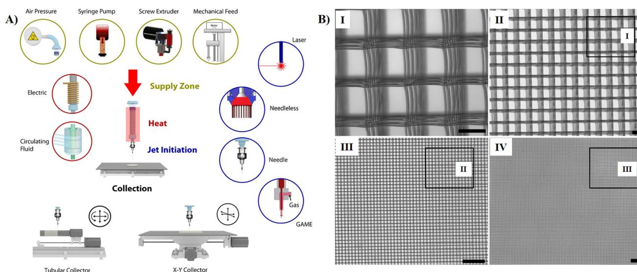
**Fig. 7** (A) Schematic of the melt ES configurations reported in the literature, (B) stereomicroscope images of a PCL scaffold fabricated using a melt ES technique. Electrospun fibers are aligned orthogonally with interfiber distance of 150 μm in both axes: scale bars for I–II and III–IV are 100 μm and 1 mm, respectively. Figures (A) and (B) have been adapted from ref. 98 with permission from Elsevier, copyright 2016.
