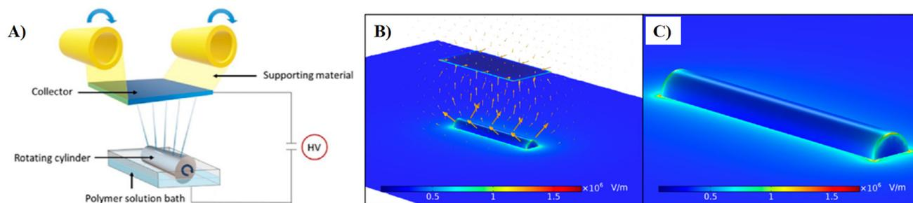
**Fig. 6** (A) Schematic representation of the 'Nanospider' technology setup with a cylinder electrode, (B) simulation of the cylinder and collecting plate configuration, (C) simulation of the electrostatic charge distribution on the electrode. Figures (A–C) have been adapted from ref. 95 with permission from Multidisciplinary Digital Publishing Institute, copyright 2021.
