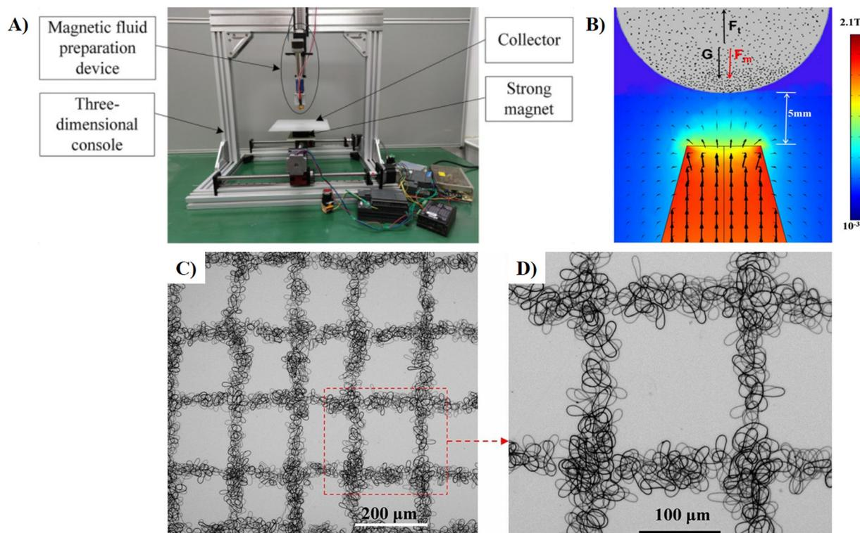
**Fig. 9** (A) The image of a homemade MMS prototype; (B) the simulation of the magnetic field in the region of 5 mm outside the nozzle tip;  $G$ ,  $F_t$ , and  $F_m$  correspond to gravitational force, surface tension, and magnetic force, respectively; (C) and (D) SEM images of patterned architecture of PS fibers at different magnifications. Figures (A–D) have been adapted from ref. 117 with permission from Nature Portfolio, copyright 2021.
