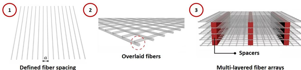
**Fig. 15** Simple scheme for assembling aligned fiber arrays into an efficient multi-layered structure using AM technologies: 1 – fabrication of aligned fiber arrays using a particular drawing method, 2 – orthogonal alignment of two fiber arrays, 3 – construction of the multi-layered fiber structure utilizing spacers that can be melt together by heat press machine. The scheme has been provided by CytoNest, Inc.
