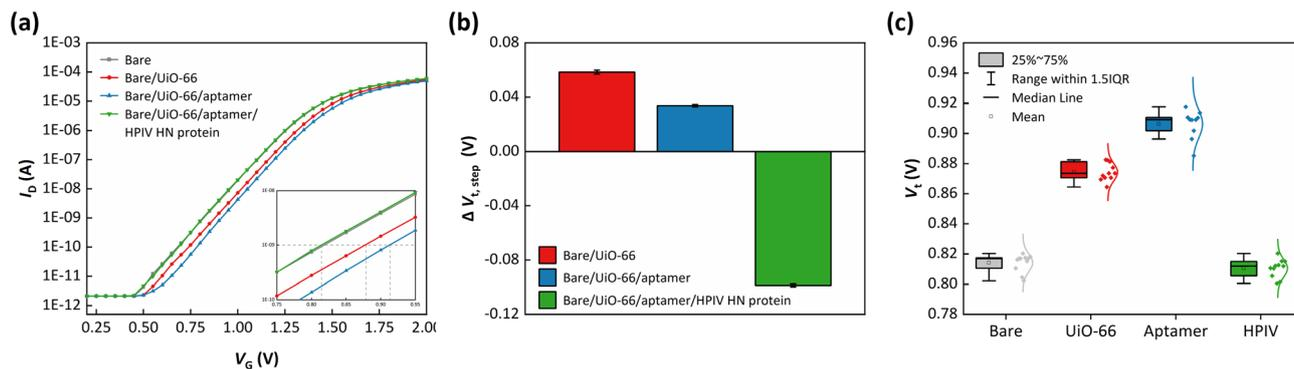
**Fig. 4** (a)  $I_D$ - $V_G$  curves from the immobilization step. (b)  $\Delta V_t$  values from the immobilization step. (c) Box plot showing the reproducibility of the  $\Delta V_t$  value according to the immobilization step. Boxplots indicate the IQR from 25 to 75% per condition, and whiskers represent  $\pm 1.5$  IQR.
