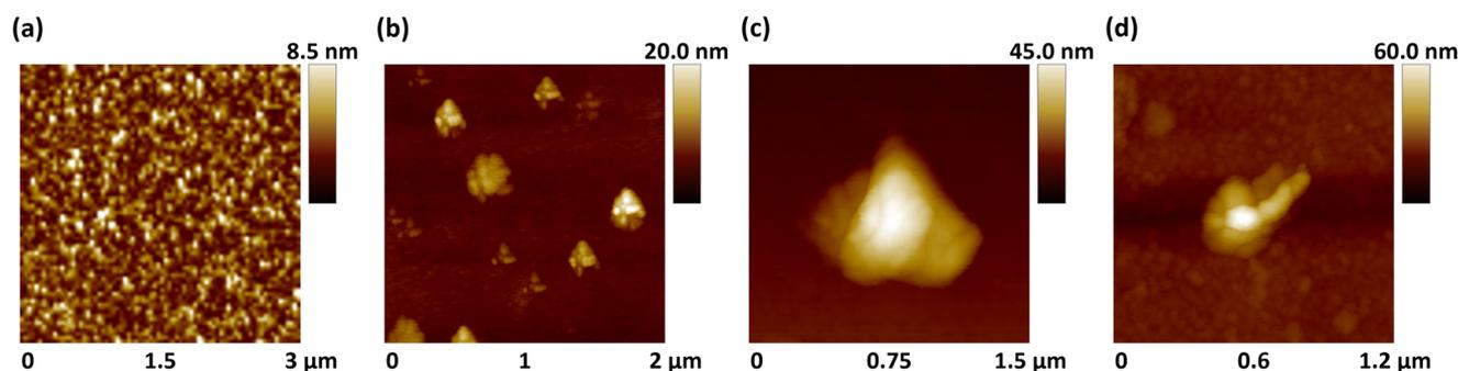
**Fig. 3** AFM images of (a) bare, (b) UiO-66-NH<sub>2</sub>, (c) UiO-66-NH<sub>2</sub>/aptamer, and (d) UiO-66-NH<sub>2</sub>/aptamer/HPIV HN protein.
