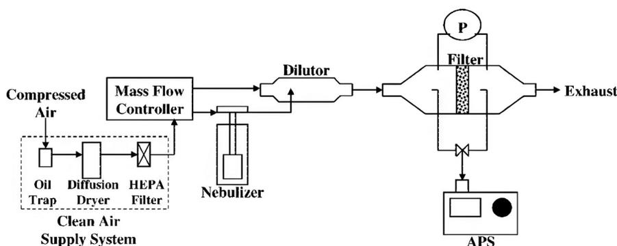
Fig. 3 Schematic diagram of experimental setup for the filtration tests.<sup>38</sup> Copyright © 2008, American Chemical Society.
