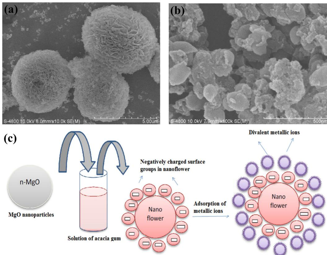
**Fig. 11** SEM images of MgO NPs samples. (a) Low magnification SEM image, (b) high magnification SEM image.<sup>146</sup> (c) Mechanism of flower-shaped MgO NPs synthesis and adsorption.<sup>134</sup> Copyright © 2015 Elsevier Ltd and Techna Group S.r.l. All rights reserved. Copyright © 2010 Elsevier B.V. All rights reserved.
