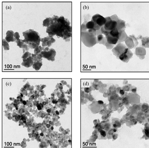
Fig. 14 HR-TEM images of biosynthesized NPs. (a) Native  $\text{TiO}_2$  NPs; (b) anatase NPs; (c) anatase and rutile NPs mix; (d) rutile NPs.<sup>183</sup> Copyright © 2014 Elsevier Ltd. All rights reserved.
