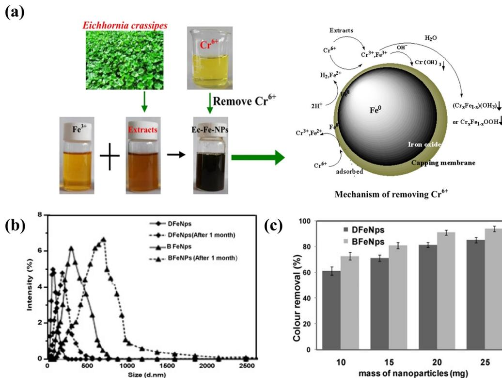
**Fig. 5** (a) The schematic diagram of Ec-Fe-NPs synthesized from *Eichhornia crassipes* leaf extracts and removal mechanism of Cr(VI).<sup>83</sup> (b) Size distributions of synthesised DFe Nps and BFe Nps. (c) The effect of Fe NPs mass on the color removal of MO dye.<sup>84</sup> Copyright © 2015 Elsevier B.V. All rights reserved.
