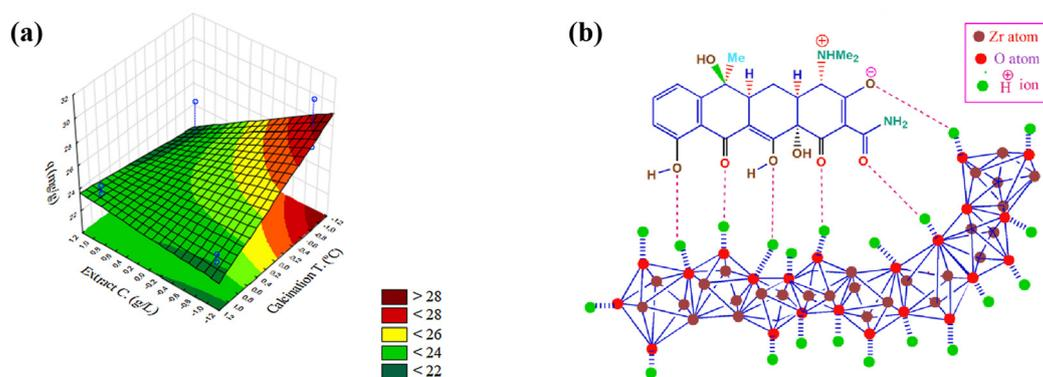
**Fig. 12** (a) The response surface with respect to the TC adsorption that relates two factors (the extract concentration and calcination temperature).<sup>17</sup> Copyright © 2019 Elsevier B.V. All rights reserved. (b) The schematic diagram for probable interaction between TC molecules and ZrO<sub>2</sub> NPs.<sup>161</sup> Copyright © 2020 Elsevier Ltd. All rights reserved.
