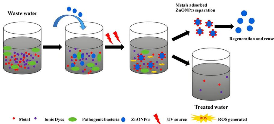
**Fig. 10** Schematic representation of how ZnO NPs can be used for systematic decontamination of wastewater containing metals, dyes, and microbes.<sup>4</sup> Copyright © 2018 Society of Chemical Industry.
