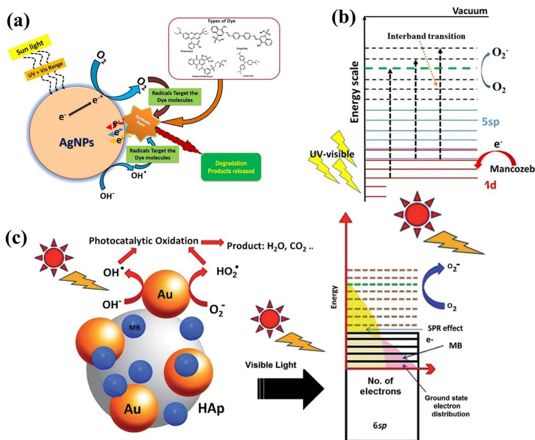
Fig. 2 (a) Schematic diagram of photocatalytic degradation dyes.<sup>13</sup> (b) Band structure of Ag NPs and its photocatalytic mechanism.<sup>39</sup> (c) Mechanism of waste removal utilizing plasmonic Au NPs based photocatalysts.<sup>58</sup> Reproduced from ref. 58 with permission from the Royal Society of Chemistry. Copyright © 2020 Elsevier B.V. All rights reserved.
