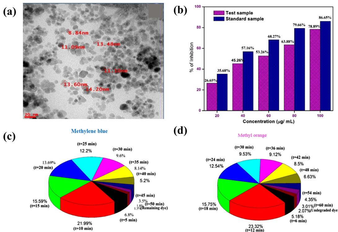
**Fig. 9** (a) TEM images of ZnO NPs at 20 nm. (b) Antioxidant activity of ZnO NPs by DPPH scavenging assay. Time-dependent photodegradation profiles (% of photodegradation vs. time) of (c) methylene blue and (d) methyl orange, presented as pie charts.<sup>16</sup> Copyright © 2016 The Society of Powder Technology Japan. Published by Elsevier B.V. and The Society of Powder Technology Japan. All rights reserved.
