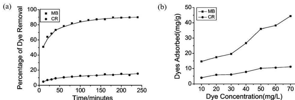
Fig. 13 The effect of experimental parameters on the adsorption of dyes (MB and CR) to  $Fe_3O_4/C$  core-shell NPs. (a) Contact time, (b) different dye equilibrium concentrations.<sup>168</sup> Copyright © Elsevier B.V. All rights reserved.
