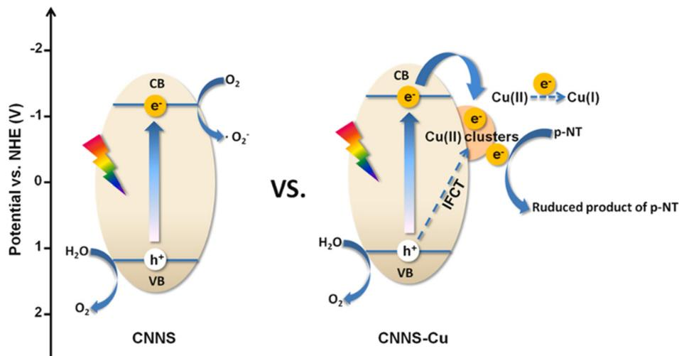
Fig. 8 The detection mechanism of *p*-NT based on CNNS-Cu 2%.<sup>100</sup> Copyright © 2022 Elsevier B.V. All rights reserved.
