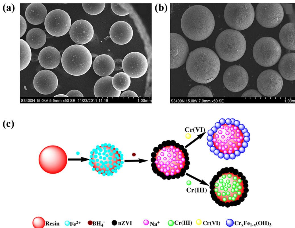
Fig. 6 (a) SEM images of resin without nZVI. (b) SEM images of resin with nZVI (c) Schematic of Cr(vi) and Cr(iii) removal mechanism by R-nZVI.<sup>93</sup> Crown Copyright © 2013 Published by Elsevier Ltd. All rights reserved.
