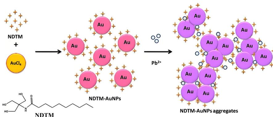
Fig. 4 Structure of NDTM and schematic representation of  $Pb^{2+}$  sensing by NDTM-AuNPs.<sup>62</sup> Copyright © 2020 Elsevier B.V. All rights reserved.
