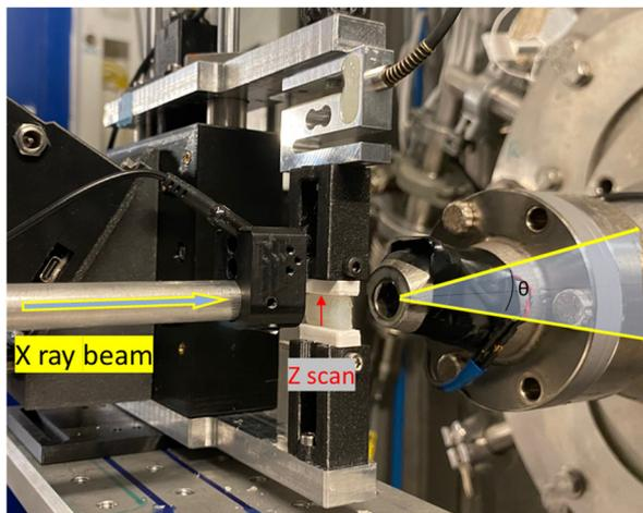
Fig. 3 Experimental set-up of the mechanical compression tests coupled with SAXS measurements.
