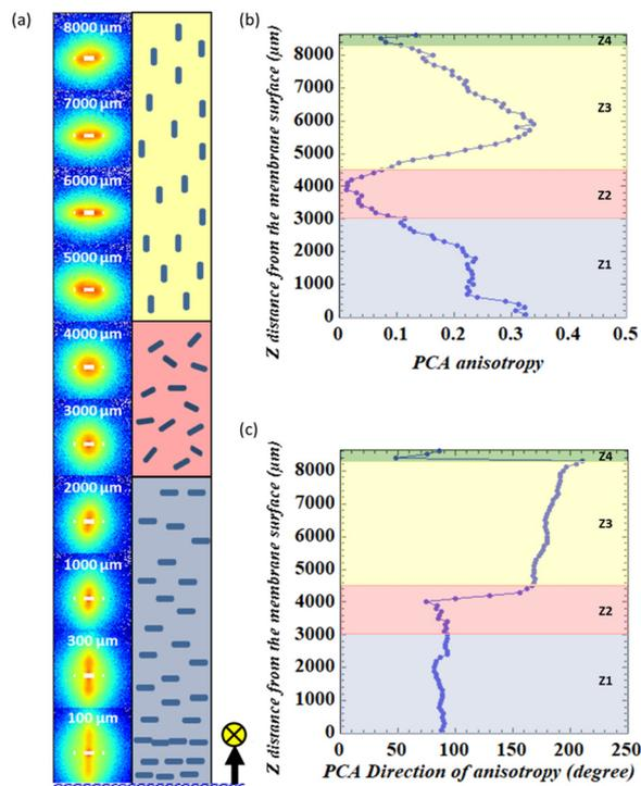
**Fig. 2** Structural characterization, anisotropy and orientation analysis of the CNC/PEGDA nanocomposite. (a) Normalized 2D SAXS patterns of the CNC/PEGDA nanocomposite, recorded *ex situ* from the membrane surface to the vibrating blade with corresponding CNC orientation. (b) PCA anisotropy and (c) direction of anisotropy in degrees as a function of the distance  $Z$  from the membrane surface.
