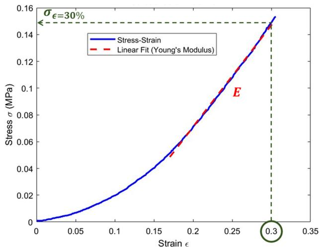
**Fig. 5** Stress–strain curve of the CNC/PEGDA nanocomposite under compression ( $\epsilon = 30\%$ ) with a Young's modulus of 0.76 MPa, calculated from the slope of the curve, and  $\sigma_{\epsilon=30\%} = 0.15$  MPa.
