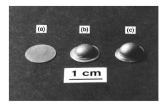
Fig. 10 Disks of an Al-Mg-Sc alloy processed by ECAP to a grain size of ~0.2 µm and then subjected to biaxial gas-pressure forming at a pressure of 10 atmospheres at 673 K: (a) untested and after (b) 30 seconds and (c) 1 minute. 105
