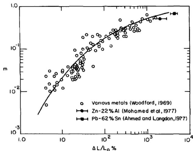
Fig. 3 Variation of strain rate sensitivity with elongation to failure<sup>13</sup> showing results for a range of materials.<sup>18–20</sup>
