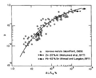
Fig. 3 Variation of strain rate sensitivity with elongation to failure 13 showing results for a range of materials. 18-20
