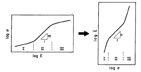
Fig. 2 Typical logarithmic plots of stress against strain rate and strain rate against stress showing the meaning of the exponents m and n.
