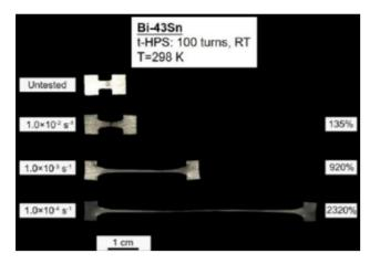
Fig. 8 An example of superplasticity in a Bi-43% Sn alloy after processing by t-HPS.<sup>87</sup>
