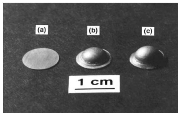
Fig. 10 Disks of an Al–Mg–Sc alloy processed by ECAP to a grain size of  $\sim 0.2 \mu\text{m}$  and then subjected to biaxial gas-pressure forming at a pressure of 10 atmospheres at 673 K: (a) untested and after (b) 30 seconds and (c) 1 minute.<sup>105</sup>
