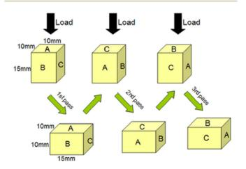
The principle of multi-directional forging or abc deformation.
