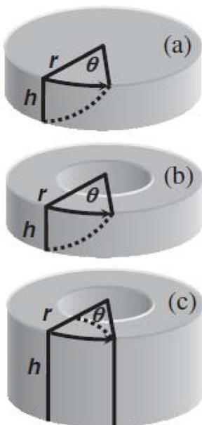
Fig. 6 Comparison of the principles of (a) HPT, (b) tube torsion/twist and (c) t-HPS.<sup>72</sup>
