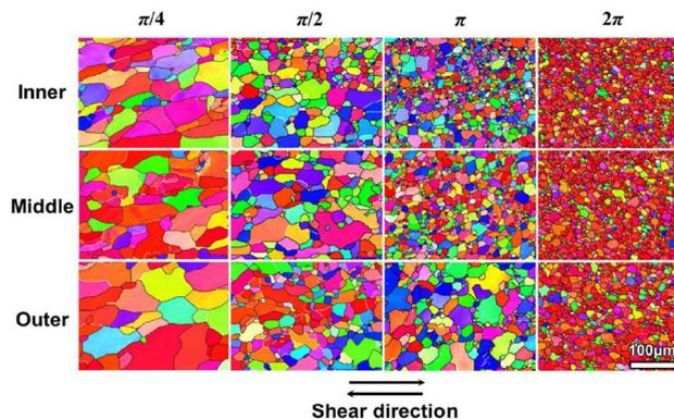
Fig. 7 Grain refinement in high-purity aluminum at the inner, middle and outer regions of the tube after processing by t-HPS through different numbers of turns.<sup>76</sup>
