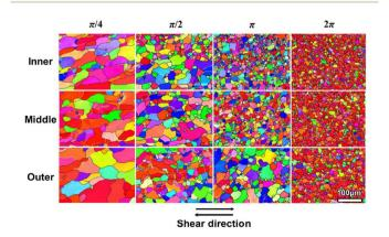
Fig. 7 Grain refinement in high-purity aluminum at the inner, middle and outer regions of the tube after processing by t-HPS through different numbers of turns.76
