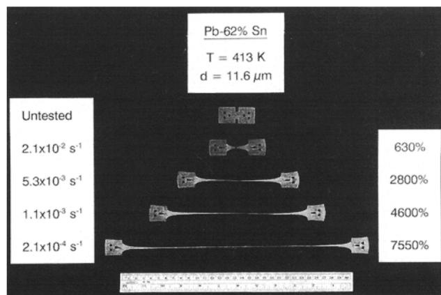
Fig. 4 An example of superplasticity in a Pb-62% Sn alloy with an elongation of 7550% at a strain rate of  $2.1 \times 10^{-4} \text{ s}^{-1}$ .<sup>26</sup>
