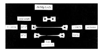
Fig. 9 An example of high strain rate superplasticity in an Al-Mg-Li-Zr alloy processed by ECAP to a grain size of ~1.2 µm and tested in tension at 623 K.<sup>104</sup>
