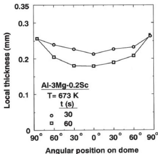
Fig. 11 The local thicknesses measured around the two deformed domes in Fig. 10 subjected to a pressure of 10 atmospheres for times of 30 and 60 seconds, respectively.<sup>105</sup>
