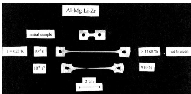
Fig. 9 An example of high strain rate superplasticity in an Al–Mg–Li–Zr alloy processed by ECAP to a grain size of  $\sim 1.2 \mu\text{m}$  and tested in tension at 623 K.<sup>104</sup>
