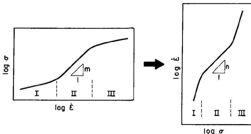
Fig. 2 Typical logarithmic plots of stress against strain rate and strain rate against stress showing the meaning of the exponents  $m$  and  $n$ .<sup>13</sup>
