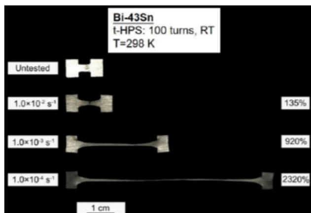
Fig. 8 An example of superplasticity in a Bi-43% Sn alloy after processing by t-HPS.<sup>87</sup>
