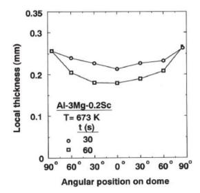
Fig. 11 The local thicknesses measured around the two deformed domes in Fig. 10 subjected to a pressure of 10 atmospheres for times of 30 and 60 seconds, respectively. 105
