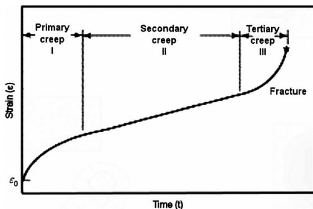
Fig. 1 A typical creep curve of strain against time showing the three regions of flow.<sup>12</sup>
