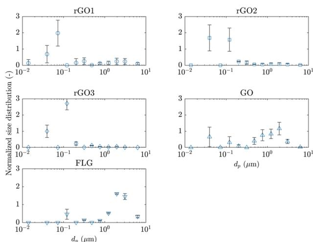
**Fig. 2** Normalised number size distributions  $f_n(d_p)$ , for dustiness-tested GRMs, showing the mean and standard deviation for each ELPI stage.<sup>60</sup> Data points near  $0.07 \mu\text{m}$  for rGO2, rGO3, and GO are suspected outliers, likely due to a single ELPI stage becoming filled or clogged with GRM.
