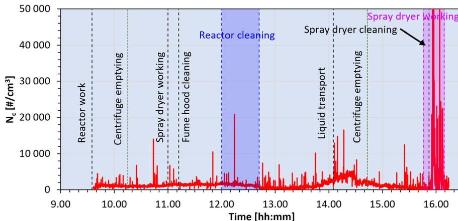
Fig. 4 Particle number concentrations ( $d_p = 10\text{--}700$  nm, DISCmini) at the worker's breathing zone during GO production over a 7-hour work shift (Scenario 6).
