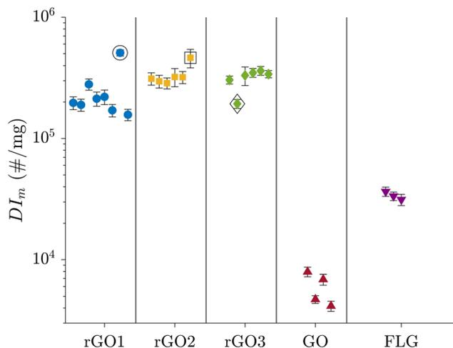
**Fig. 1** Number-based dustiness indices for five GRMs from individual dustiness tests ( $n = 27$ ), based on UCPC data ( $d_p = 2.5 \text{ nm} - 1 \mu\text{m}$ ). Error bars indicate the limits from the propagation of uncertainty (maximal error). Outliers, encircled on the plot, likely result from measurement inconsistencies, such as partial clogging of sampling lines or the cyclone with GRM, affecting sampling flows or releasing GRM.
