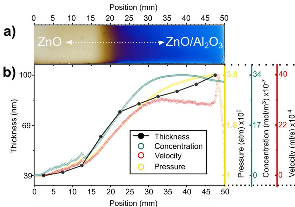
Fig. 4 (a) The image of combinatorial nanolaminate film ZnO/Al<sub>2</sub>O<sub>3</sub>. (b) Ellipsometry thickness measurements (solid dots) and CFD simulation averaged profiles (hollow dots) on the substrate surface sequentially; velocity, concentration and pressure profiles, as a function of sample position.
