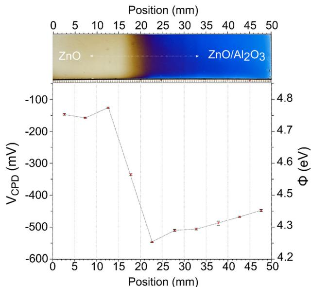
**Fig. 8** The contact potential difference, represented on the left y-axis, and the calculated work function values, displayed on the right y-axis, were systematically measured at various points on the investigated samples.
