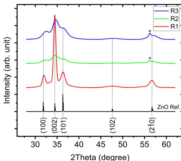
**Fig. 6** GI-XRD patterns of the thin film sample at incident angles of 0.34°. The diffraction peaks correspond to the crystalline phases present in the surface layer, with a notable decrease in the (002) peak of ZnO by increasing Al<sub>2</sub>O<sub>3</sub> composition, indicating a reduction of crystalline quality. PDF Card – 04-020-0364 used as a reference ZnO spectra the intensity multiplied fifty times.
