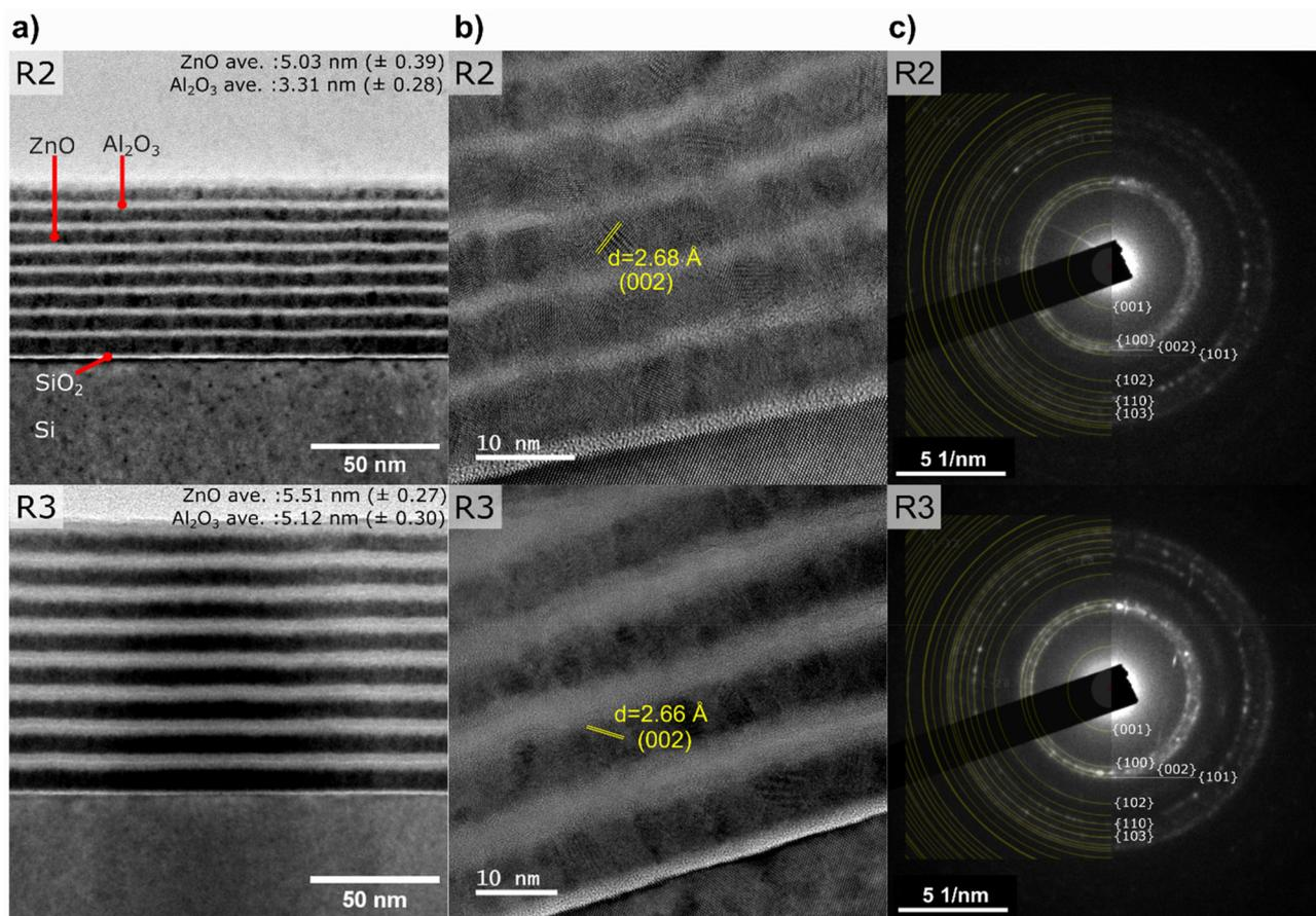
**Fig. 7** TEM analysis of ZnO/Al<sub>2</sub>O<sub>3</sub> nanolaminate films. (a) TEM cross-sectional image shows the ZnO/Al<sub>2</sub>O<sub>3</sub> bilayer deposited with eight super-cycle. ZnO and Al<sub>2</sub>O<sub>3</sub> sublayers have been annotated (b) HR-TEM image showing lattice fringes with a measured spacing of 2.7 Å for ZnO film. (c) SAED pattern indexed to the ZnO (PDF Card – 04-020-0364).
