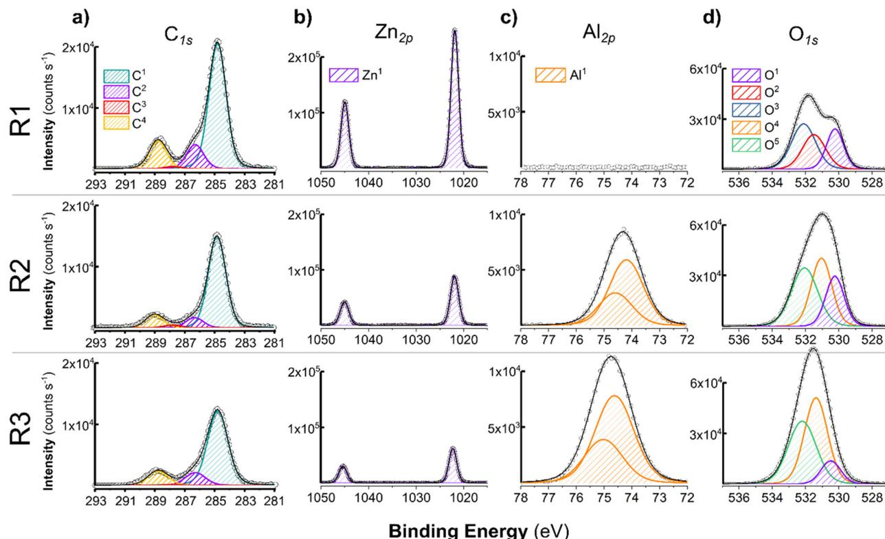
**Fig. 3** HR-XPS spectra with fitted contributions; (a)  $C_{1s}$ , (b)  $Zn_{2p}$ , (c)  $Al_{2p}$ , and (d)  $O_{1s}$  regions obtained for SALD-deposited films. The black dots represent experimental data, while the solid black line corresponds to the fitted envelope.
