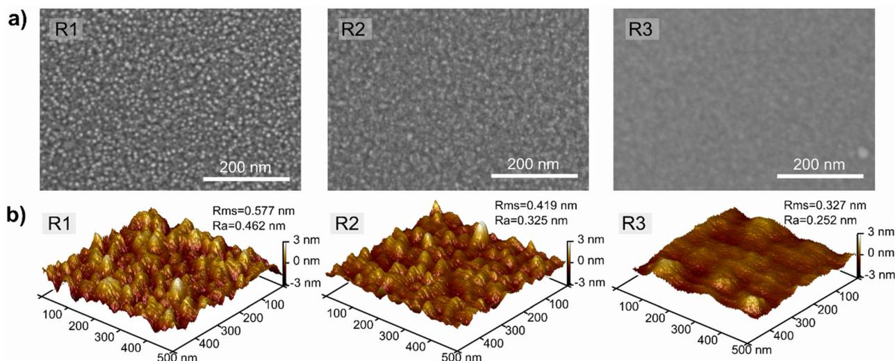
**Fig. 5** (a) Top-view SEM images showing the surface morphology of nanolaminate ZnO/Al<sub>2</sub>O<sub>3</sub> film from different regions R1, R2, and R3. (b) AFM images displaying the surface roughness over 500 × 500 nm<sup>2</sup> areas of the same regions. Both RMS and *R<sub>a</sub>* roughness values are included.
