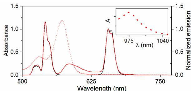
Fig. 2 Absorption spectrum of UC@RB (red dashed line) and normalized UC luminescence spectra ( $\lambda_{\text{exc}} = 980$  nm) of UC@BF<sub>4</sub> (black line) and UC@RB (red line) in DMF. Inset: Absorbance in the range 950–1050 nm.
