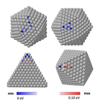
Fig. 2 Energy differences between different adatom positions. In order from the up and left: chiral icosahedron, Mackay icosahedron, tetrahedron and octahedron. In the tetrahedron, the four vertices are removed, as in the MD simulations. For each structure, we show the inequivalent adsorption sites (small spheres on the nanoparticle surface), coloured according to their energy difference from the most favourable site on that structure.
