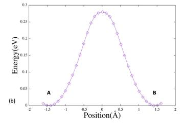
Fig. 3 Edge crossing by jump on the Mackay icosahedron. (a) Adsorption sites before and after the crossing of the edge by jump diffusion. (b) Energy profile of the diffusion process, estimated by the drag method. The energy barrier is 0.27 eV.
