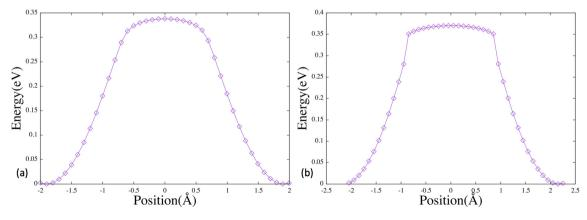
Fig. 5 Edge crossing by jump on the octahedron and tetrahedron. Energy profiles for edge crossing diffusion by jump on the (a) octahedron and (b) tetrahedron, estimated by the drag method. The energy barriers are 0.33 and 0.38 eV, respectively.
