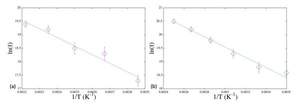
Fig. 8 Arrhenius plot for inter-facet diffusion by jump on the Mackay and chiral icosahedron. (a) Mackay icosahedron. Energy barrier and pre-exponential factor are  $\Delta E = (0.28 + 0.03)$  eV and  $A = 3.6 \times 10^{11}$ . (b) Chiral icosahedron. Energy barrier and pre-exponential factor are  $\Delta E = (0.16 + 0.01)$ eV and  $A = 9 \times 10^{10}$ . Frequencies f are in s<sup>-1</sup>.
