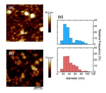
Fig. 1 AFM topography images of P3HT NPs deposited on a silicon wafer. (a) Miniemulsion NPs and (b) flash NPs. (c) Particle size histograms for miniemulsion NPs (blue histogram) and flash NPs (red histogram).
