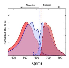
Fig. 3 Absorption (UV-Vis) and emission (photoluminiscence) spectra of flash P3HT NPs (red) and miniemulsion P3HT NPs (blue). Excitation wavelength 555 nm. The curves were normalized to the maximum intensity.
