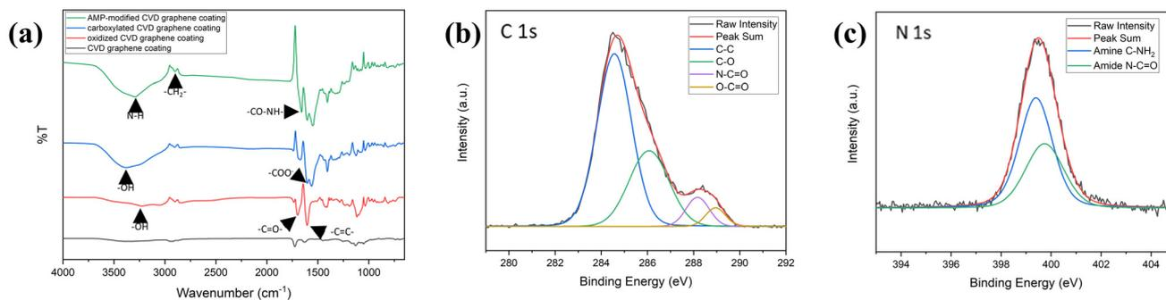
**Fig. 4** Characterization of AMP-modified CVD graphene coating. (a) FTIR spectra of CVD graphene coating before and after each step. (b) XPS C 1s narrow scan and (c) XPS N 1s narrow scan of AMP-modified G-PDMS.
