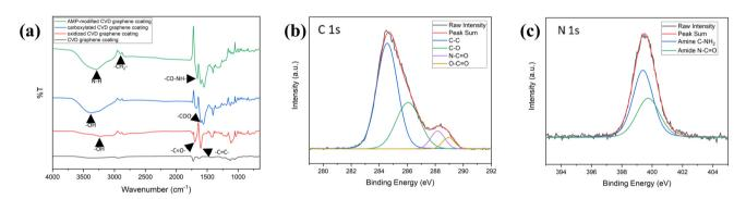
Fig. 4 Characterization of AMP-modified CVD graphene coating. (a) FTIR spectra of CVD graphene coating before and after each step. (b) XPS C 1s narrow scan and (c) XPS N 1s narrow scan of AMP-modified G-PDMS.
