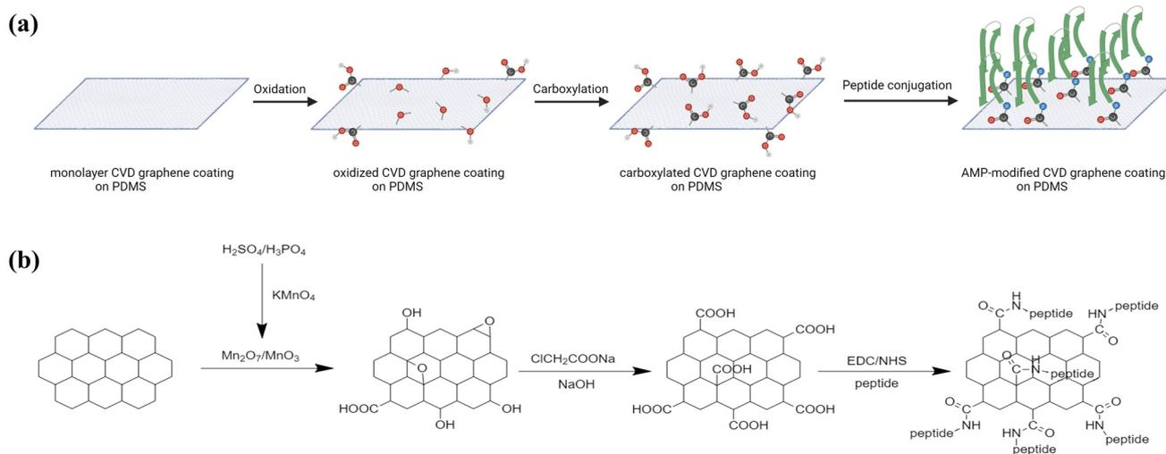
**Fig. 3** Preparation of AMP-modified CVD graphene coating. (a) Schematic showing the covalent conjugation of AMP on CVD graphene coating. (b) Synthesis route of AMP-modified CVD graphene coating: step 1 oxidation to add oxygen functional groups; step 2 carboxylation to convert the oxygen functional groups to carboxyl groups; and step 3 peptide conjugation to conjugate the peptide through the amide bond.
