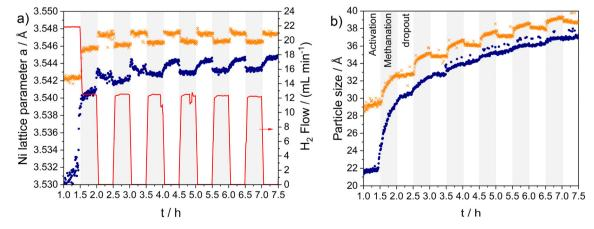
Fig. 1 (a) Evolution of lattice parameters for the Ni@SBa150 (blue circle) and SPP2080-IMRC (orange crosses) catalysts during the experiment. The H<sub>2</sub> flow is presented in red. (b) Evolution of the particle size for the two catalysts during methanation (gray area) and H<sub>2</sub> dropout (white area). The values were obtained by PDF fitting.
