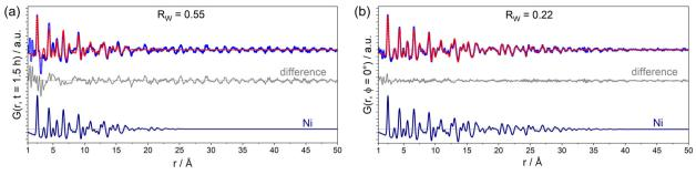
Fig. 5 PDF refinement of d-PDF (a) and PSD data (b) using Nifcc as a single phase. Experimental PDF data are shown as blue circles, the fitted calculated PDF is shown as a red line, and the difference curve is shown in grey (offset), with the goodness-of-fit, Rw, in each panel.
