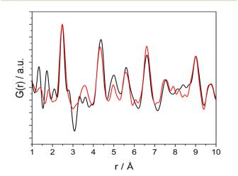
Fig. 4 Comparison between the d-PDF (black) and the PSD transformed ME-PDF data at the in-phase angle  $\phi^{\rm PSD}$  = 0° (in red) for the SPP2080-IMRC sample in the r range between 1 and 10 Å. The d-PDF pattern reported is from the first dataset right after the activation process as soon the methanation starts (t = 1.5 h). The data shown are normalized to the most intense peak (2.48 Å) for better comparison.
