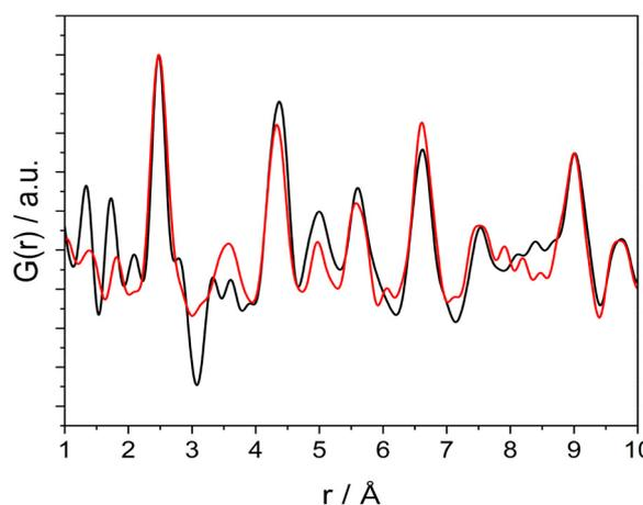
**Fig. 4** Comparison between the d-PDF (black) and the PSD transformed ME-PDF data at the in-phase angle  $\phi^{\text{PSD}} = 0^\circ$  (in red) for the SPP2080-IMRC sample in the  $r$  range between 1 and 10 Å. The d-PDF pattern reported is from the first dataset right after the activation process as soon the methanation starts ( $t = 1.5$  h). The data shown are normalized to the most intense peak (2.48 Å) for better comparison.
