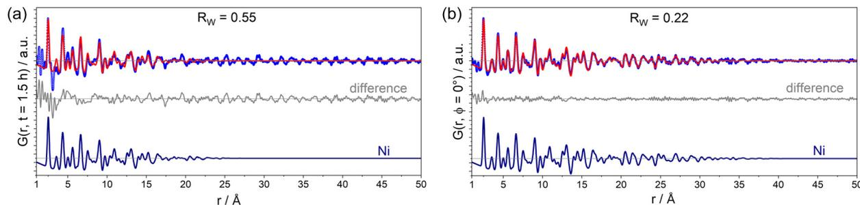
**Fig. 5** PDF refinement of d-PDF (a) and PSD data (b) using  $\text{Ni}_{\text{fcc}}$  as a single phase. Experimental PDF data are shown as blue circles, the fitted calculated PDF is shown as a red line, and the difference curve is shown in grey (offset), with the goodness-of-fit,  $R_W$ , in each panel.
