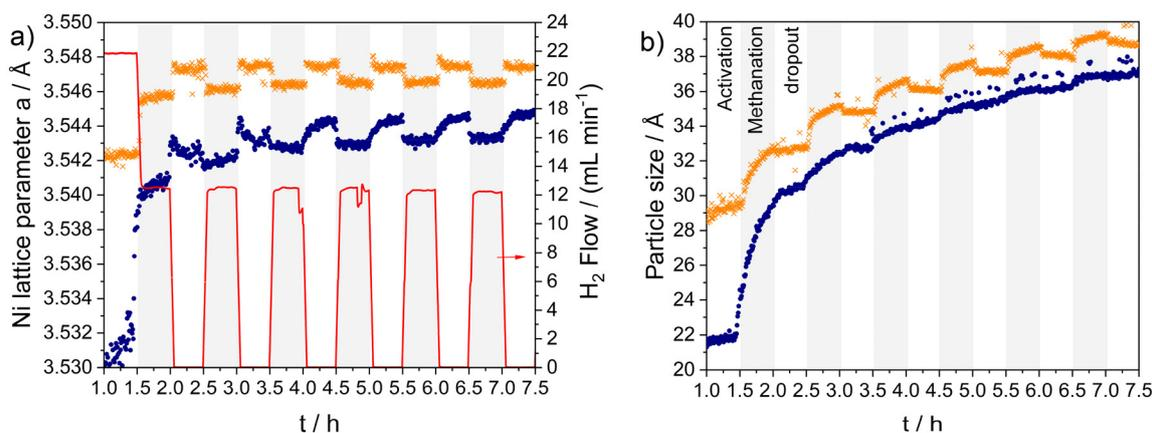
**Fig. 1** (a) Evolution of lattice parameters for the Ni@SBa150 (blue circle) and SPP2080-IMRC (orange crosses) catalysts during the experiment. The H<sub>2</sub> flow is presented in red. (b) Evolution of the particle size for the two catalysts during methanation (gray area) and H<sub>2</sub> dropout (white area). The values were obtained by PDF fitting.
