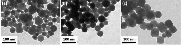
Fig. 6 TEM images of the Ag nanoparticles resulting from (a) a synthesis with Ag acetate as precursor instead of AgNO<sub>3</sub>, (b) the standard synthesis, and (c) a synthesis with additional  $NH_4NO_3$ .
