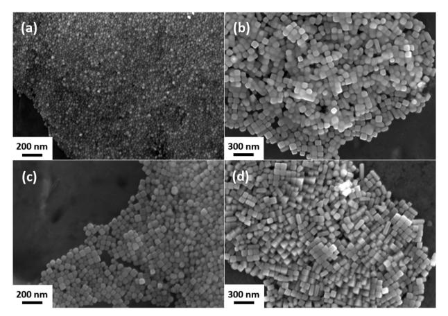
Fig. 1 SEM images of Aq nanoparticles synthesized with and without exposure to different metal surfaces: (a) no metals used (glass thermometer), (b) steel thermometer used, (c) V4A steel capillary used with a glass thermometer, and (d) FeCl<sub>3</sub>·6H<sub>2</sub>O powder used with a glass thermometer.
