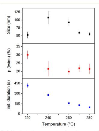
Fig. 5 Plots showing the temperature dependency of the nanoparticle edge lengths (top), the percentage of (multiply) twinned nanoparticles (p = percentage of MT crystals in relation to the total amount of Agnanoparticles) (middle), and the duration of the color change of the initial reaction (bottom).
