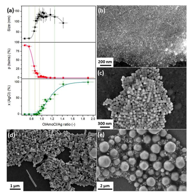
Fig. 3 (a) Influence of the Cl: Ag ratio on the edge length of the nanoparticles (top), on the occurrence of twinned nanoparticles (p = percentageof MT crystals in relation to the total amount of Ag nanoparticles) (middle), and the mass proportion of AgCl relative to Ag (bottom) in the final product. The green vertical lines mark the CI: Ag ratios used in the synthesis of the particles shown in the exemplarily SEM images are (b) 0.75, (c) 0.85, (d) 0.93, and (e) 1.25.
