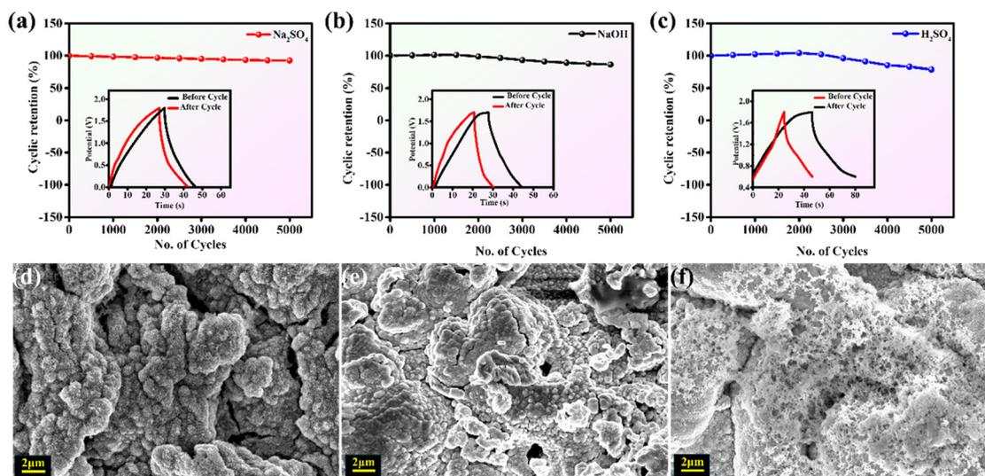
**Fig. 8** (a) Cycling stability curve with the inset showing the first and last GCD cycles at 8 mA cm<sup>-2</sup>, and the corresponding FESEM images of the WSe<sub>2</sub>@graphite electrode after 5000 cycles with different electrolytes: (a and d) Na<sub>2</sub>SO<sub>4</sub>, (b and e) NaOH, and (c and f) H<sub>2</sub>SO<sub>4</sub>.
