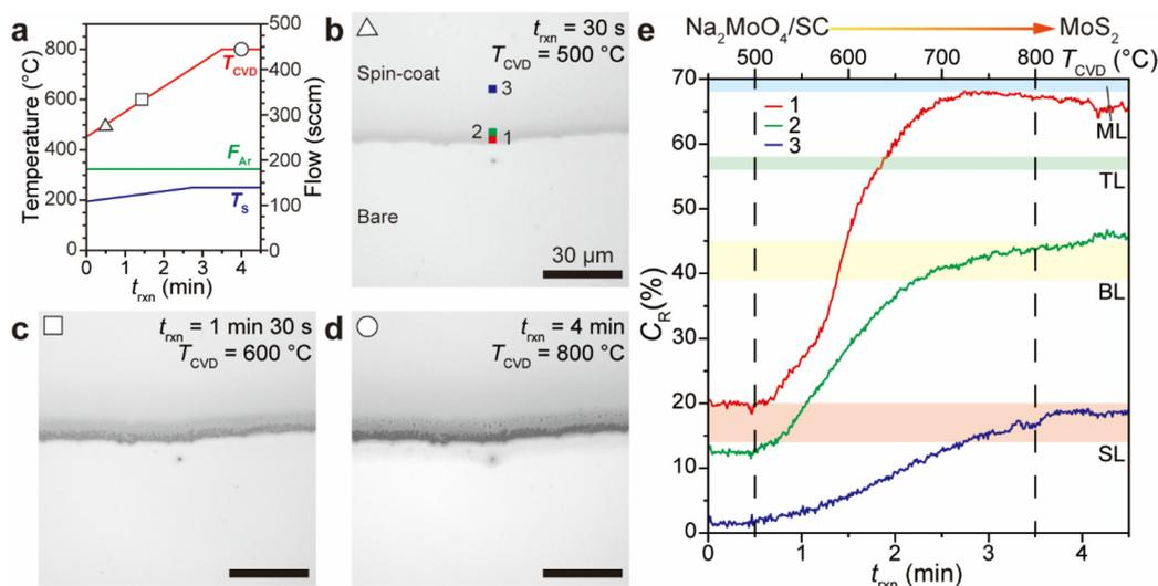
**Fig. 5** Growth kinetics of the continuous MoS<sub>2</sub> film observed using an ICVDM. (a) Programming parameter ( $T_{\text{CVD}}$ ,  $T_s$ , and  $F_{\text{Ar}}$ ) profiles during the ICVDM reaction. Real-time optical images of the MoS<sub>2</sub> film at  $t_{\text{rxn}} =$  (b) 30 s, (c) 1 min 30 s, and (d) 4 min. (e)  $C_R$  trends of the positions in the optical images in (b) according to  $t_{\text{rxn}}$  and  $T_{\text{CVD}}$ .
