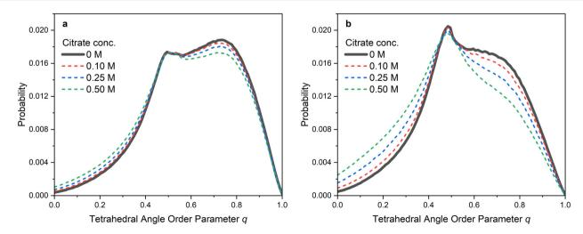
Fig. 5 Distributions of the tetrahedral order parameter q, obtained from simulations a. in bulk phase and b. in the region close to the interface at various citrate concentrations.
