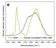
Fig. 4 The bulk and solute-correlated spectra for aqueous citrate solutions of a. 1 mM, b. 5 mM, c. 10 mM, d. 100 mM and e. 1000 mM strengths.
