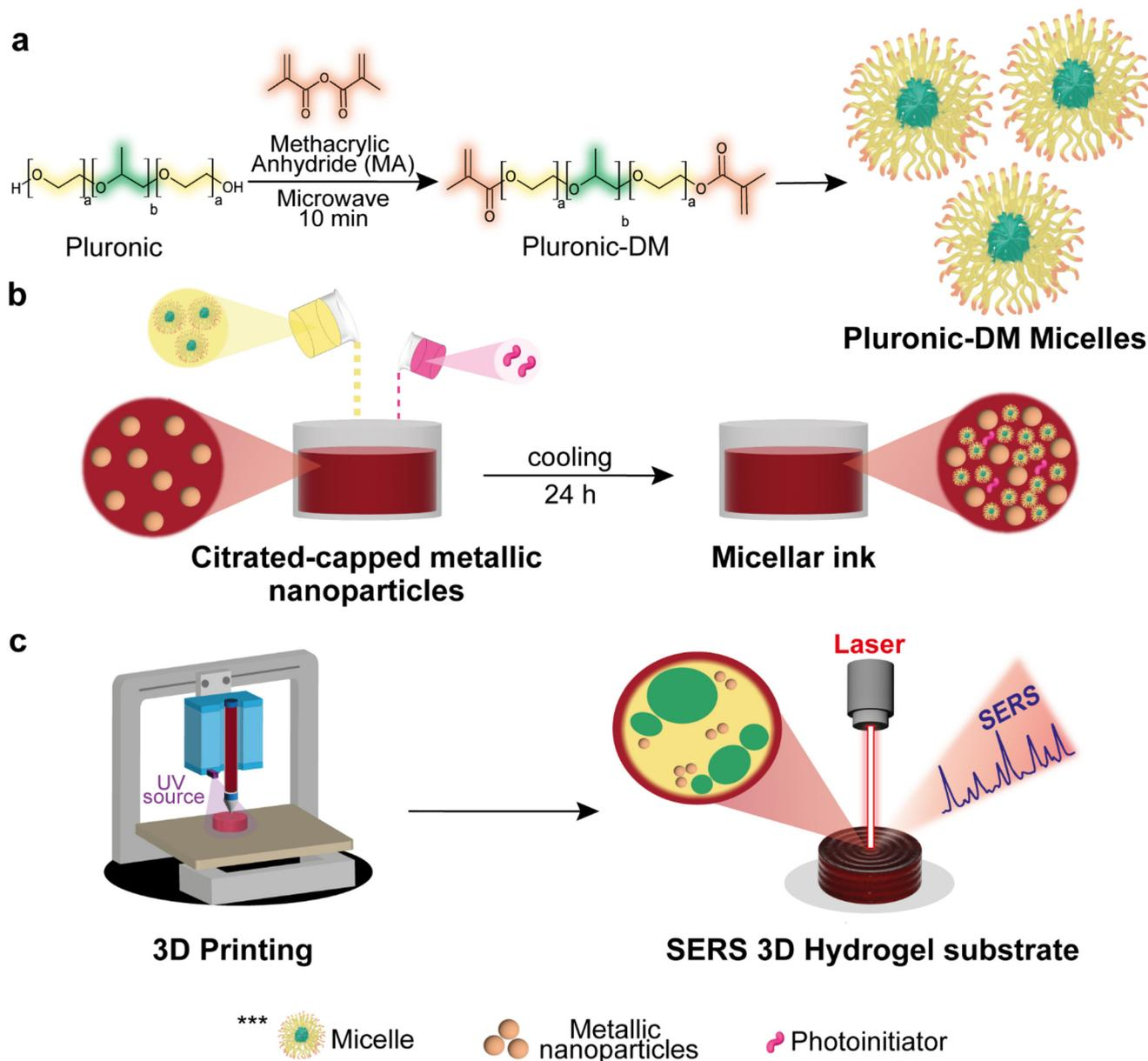
**Fig. 1** Schematic illustration of (a) microwave-assisted methacrylation of pluronic F127 and micelle formation, (b) micellar ink preparation, (c) 3D printing of SERS hydrogel substrates with micellar photocrosslinkable plasmonic inks (AuNPs and AgNPs).
