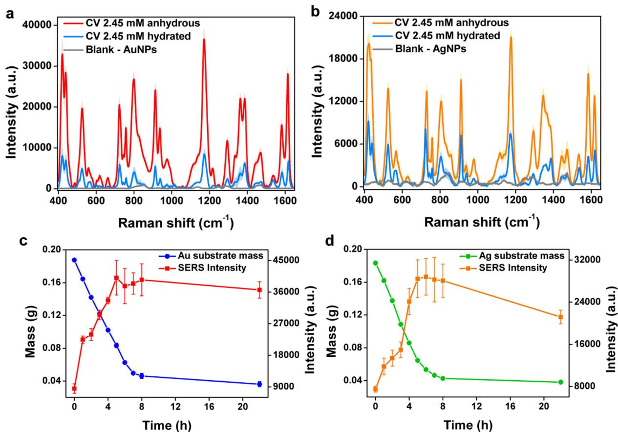
Fig. 3 SERS spectra of 2.45  $\mu\text{M}$  crystal violet in anhydrous and fully hydrated SERS substrates made of (a) AuNPs and (b) AgNPs. Temporal assessment of water loss and SERS intensity at  $1173\text{ cm}^{-1}$  for the 3D-printed plasmonic hydrogels made of (c) AuNPs and (d) AgNPs. Time = 0 h represents the 3D-printed substrates at the state of maximum swelling/hydration.
