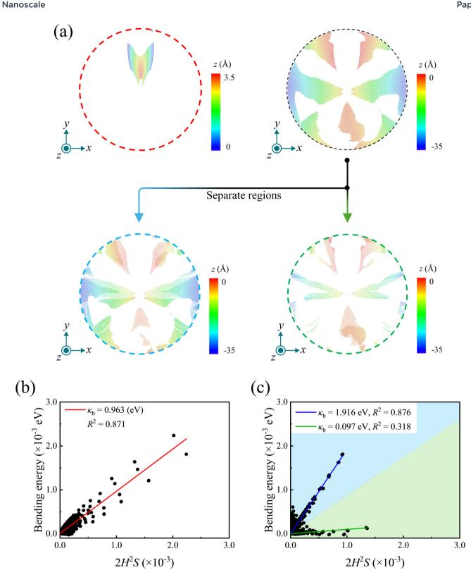
Fig. 7 (a) Atomic diagram when the regions are divided. Fitting after cutoff due to stretching energy: (b)  $z \ge 0$  region, and (c) z < 0 region.
