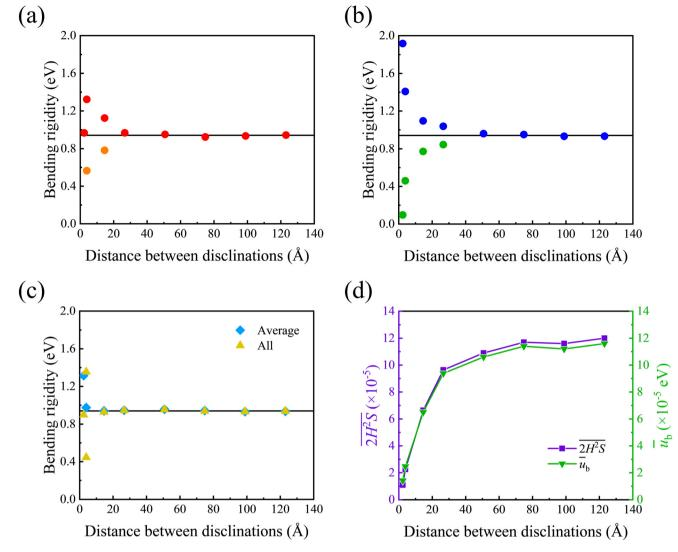
Fig. 10 Relationship between distance between disclinations and bending rigidity of SDD: (a)  $z \ge 0$ , and (b) z < 0. (c) Overall fitting bending rigidity and weighted-average bending rigidity. (d) Relationship between distance between disclinations and  $2H^2S$  or bending energy per atom. Bars represent average values per atom.
