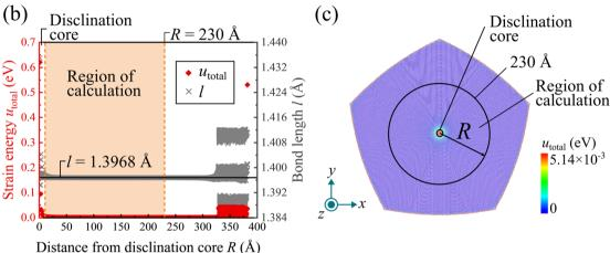
Fig. 3 (a) Surface approximation. (b) Relationship between the distance from the defect core and strain energy and bond length, and (c) strain-energy distribution diagram of the GS with the positive disclination monopole.
