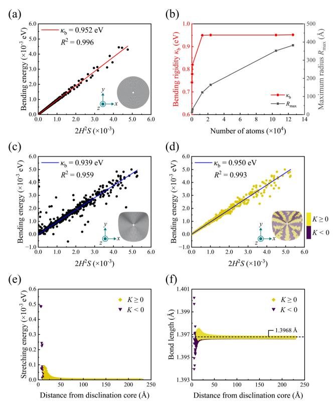
Fig. 4 Results for positive disclination: (a) Relationship between 2H<sup>2</sup>S and bending energy and (b) effect of size on bending rigidity. Results of negative disclination: (c) Relationship between 2H<sup>2</sup>S and bending energy. (d) Fitting only atoms of positive Gaussian curvature. (e) Plot of stretching energy with distance from disclination core. (f) Plot of bond length per atom with distance from disclination core. The black line is the ideal GS bond length (l = 1.397 Å).
