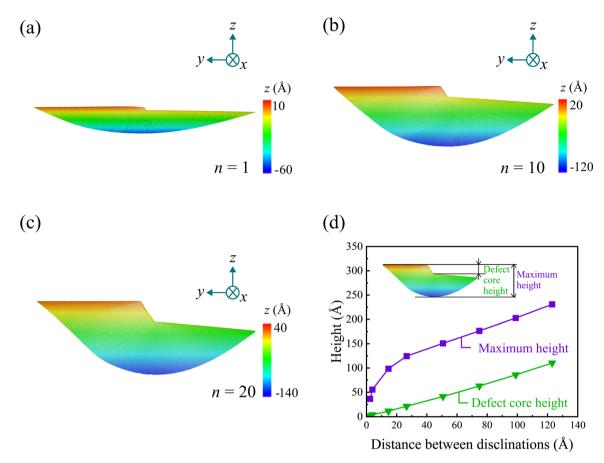
Fig. 8 SDD models and height: number of six-membered rings between the disclinations is (a) n = 1, (b) n = 10, and (c) n = 20. (d) Relationship between the number of six-membered rings between the disclinations and the height in the z-direction (purple: maximum height, green: defect cores height).
