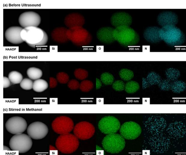
**Fig. 5** High-angle annular dark-field-scanning transmission electron microscopy (HAADF-STEM) and energy dispersive X-ray mapping (EDS) to show distribution of silicon (Si), oxygen (O) and nitrogen (N) of **m-CPCCSiO<sub>2</sub>** (a) pre-ultrasound in water, (b) post ultrasound (P20, 10 min) in water and (c) after stirring in methanol (72 h). HAADF-STEM magnification from 190–540 kX, 300 kV electron beam.
