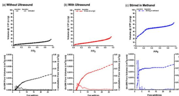
**Fig. 6** Nitrogen adsorption–desorption isotherms at 77 K and calculated pore size distribution of **m-CPC@SiO<sub>2</sub>** (a) untreated (b) after treatment with US (10 min, P10) and (c) after stirring in methanol for 72 h.
