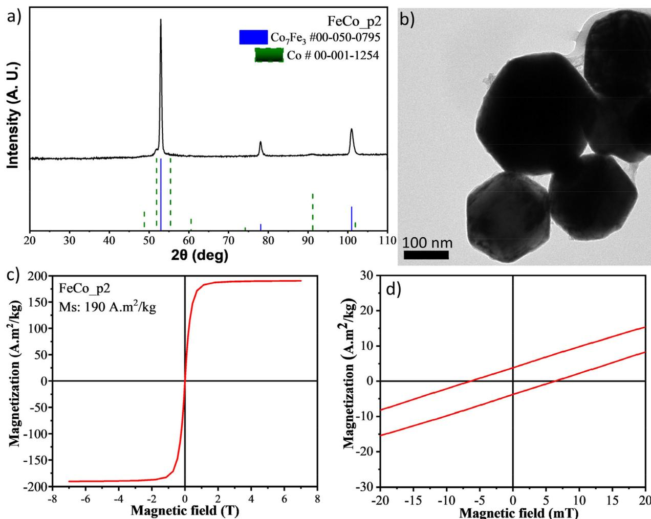
Fig. 8 (a) XRD measurement, (b) TEM image and (c) SQUID measurement for the sample FeCo\_p2, (d) a close look of the M-H plot between  $-20$  and  $20$  mT.
