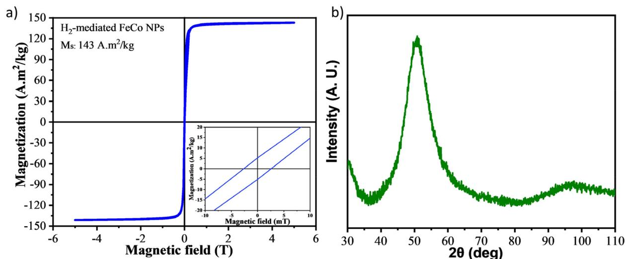
Fig. 10 (a) SQUID measurement recorded at room temperature and (b) XRD diffractogram for the H<sub>2</sub>-mediated FeCo NPs. The inset in (a) shows a zoom in of low values of magnetic field.
