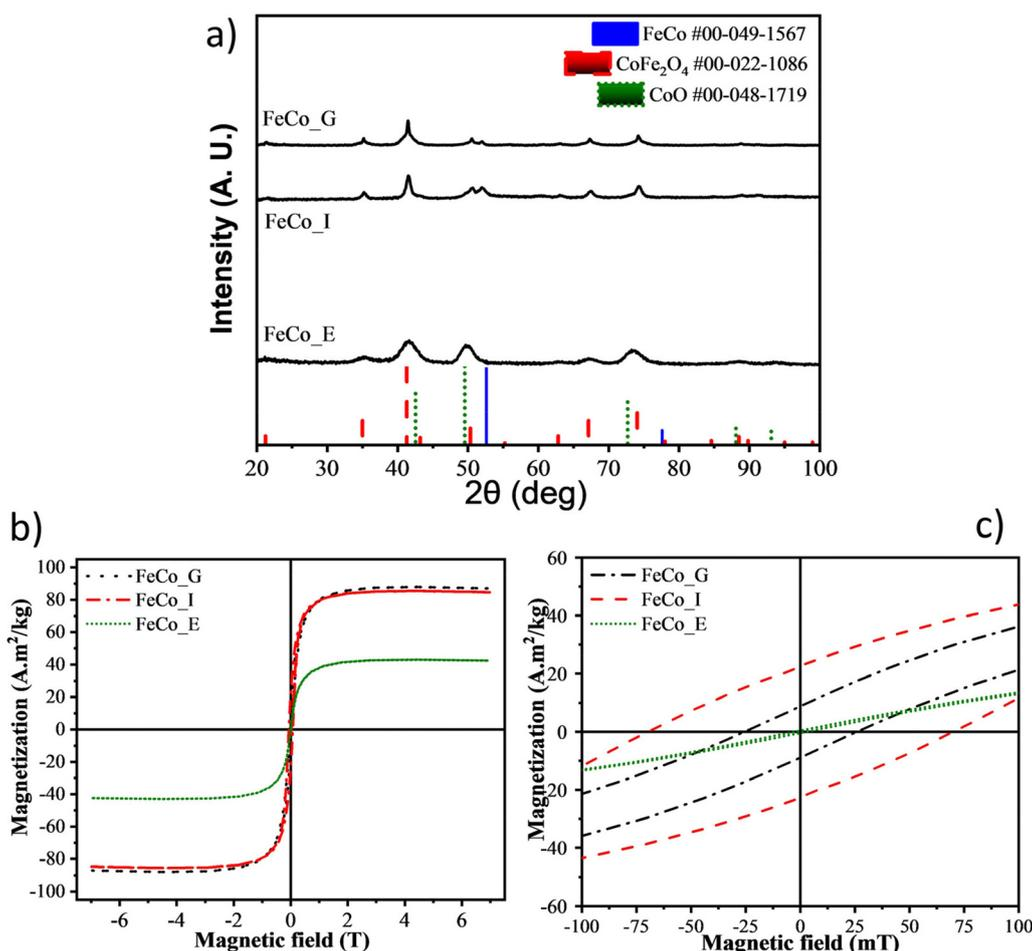
Fig. 4 XRD diffractograms (a) and SQUID measurements (b) for the three samples prepared with M-acac precursors. Graph c is a zoom in of hysteresis loops between  $-100$  and  $100$  mT.
