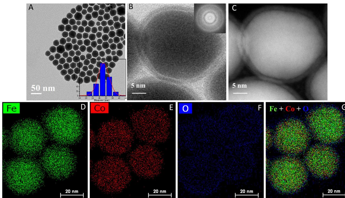
Fig. 9 Electron microscopy characterization of the H<sub>2</sub>-produced FeCo NPs: TEM image and size histogram as inset (A); HRTEM image with the SAED pattern as inset (B); HAADF-STEM image (C); HAADF-STEM-EDX elemental mapping for the different elements (D–F); and overlapping maps (G).
