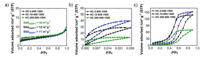
Fig. 1 Sorption isotherms of the investigated glucose-derived hard carbons after final carbonization: (a) N<sub>2</sub> physisorption isotherms at 77 K; (b) CO<sub>2</sub> physisorption isotherms at 273 K; (c) H<sub>2</sub>O vapour physisorption isotherms at 298 K.
