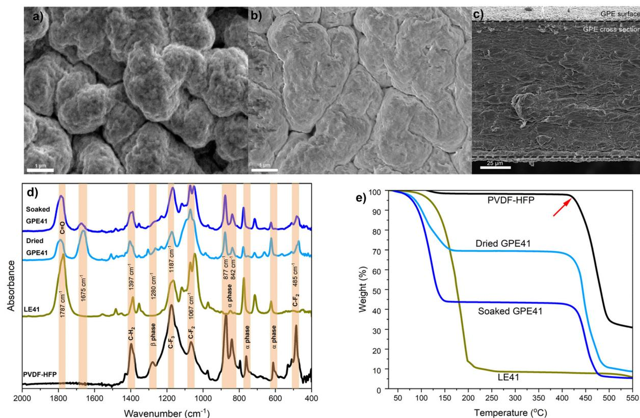
**Fig. 1** SEM image of (a) dried GPE41 and (b) soaked GPE41. (c) SEM image of the cross-section of soaked GPE41. (d) FTIR spectra of pristine PVDF-HFP, LE41, and GPE41 after vacuum-drying and GPE41 after soaking in LE41. (e) TGA of pristine PVDF-HFP, dried GPE41, soaked GPE41 and LE41.
