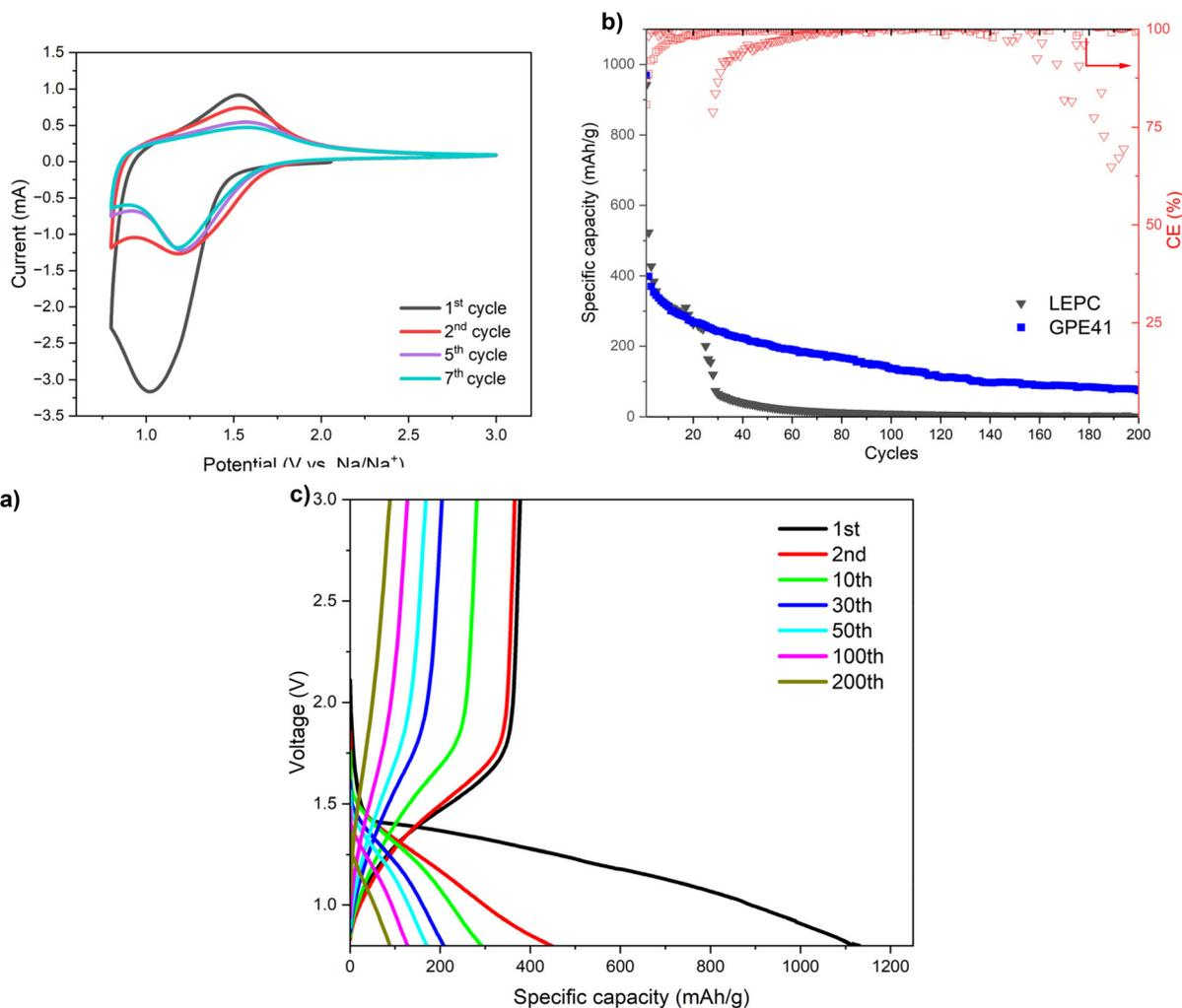
Fig. 4 (a) Cyclic voltammetry of Na|GPE41|SPAN with 0.1 mV s<sup>-1</sup> scan rate and 0.8 V–3 V potential window. (b) Capacity versus cycle from the galvanostatic charge and discharge test of full-cell Na|GPE41|SPAN at 0.1C. (c) Voltage profiles of full-cell Na|GPE41|SPAN long cycle at 0.1C.
