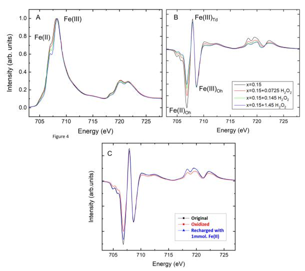
Fig. 3 XA (A) and XMCD (B) spectra for x = 0.15 nanoparticles before and after reaction with different concentrations of H<sub>2</sub>O<sub>2</sub>. (C) XMCD spectra for the x = 0.15 sample before oxidation, after oxidation with 0.0725 H<sub>2</sub>O<sub>2</sub> and after resupply with 1 mmol FeCl<sub>2</sub>.
