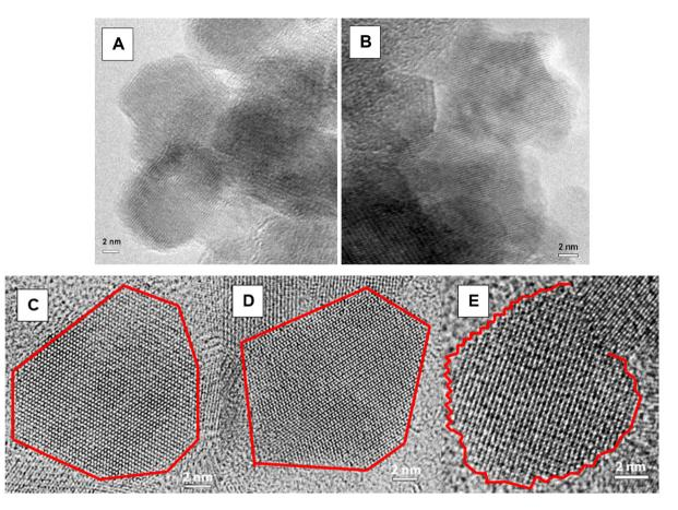
Fig. 1 TEM of x = 0.15 (A) before and (B) after oxidation with  $H_2O_2$ ; (C) x = 0.15 as-synthesized, euhedral with straight edges, with a diameter of  $\sim$ 9.5 nm; (D) x = 0.15 oxidized, euhedral with straight edges and a diameter of  $\sim$ 8.8 nm; (E) x = 0.15 recharged, rounded, rough edges, with a diameter of  $\sim$ 9.6 nm.
