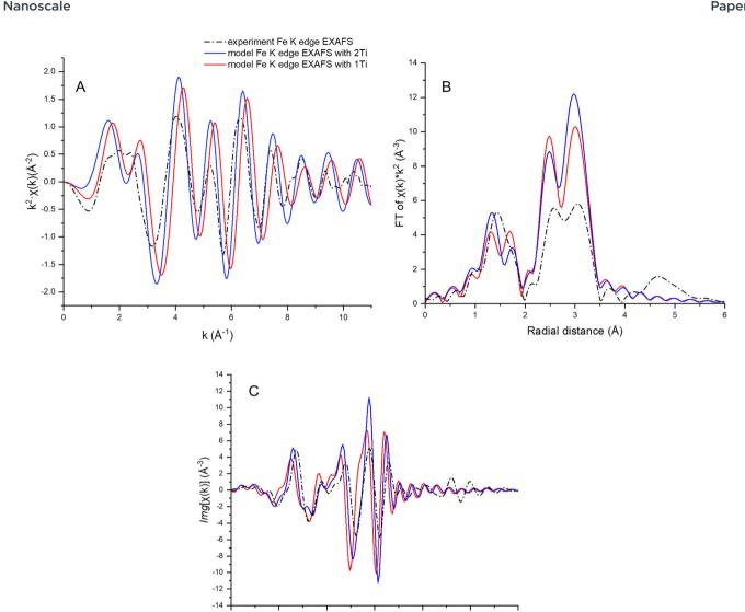
Fig. 5 Fe K-edge (A) EXAFS data, (B) Fourier transform magnitude, and (C) imaginary part for as-synthesized titanomagnetite (x = 0.15) nanoparticles (dotted black line); calculated Fe K-edge EXAFS for magnetite cell with one substituting octahedral Ti atom (red) and with two substituting octahedral Ti atoms (blue).
