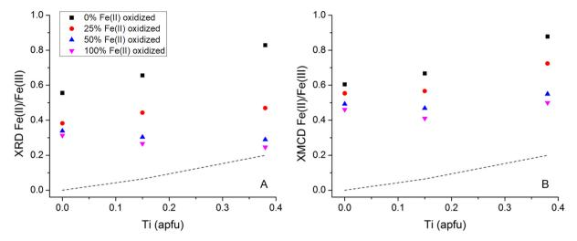
Fig. 2 Change in (A) XRD-derived Fe(ii)/Fe(iii) ratio and (B) XMCD-derived Fe(ii)/Fe(iii) ratio, as a function of x, with a theoretical 0%, 25%, 50%, and 100% of the Fe(ii) oxidized using different concentrations of  $H_2O_2$  (exact volumes of  $H_2O_2$  used are provided in Table 2). The dashed line represents the  $Fe^{2+}$  in the  $Fe_{3-x}Ti_xO_4$  structure to charge balance Ti(iv) (Worm and Banerjee, 1984).
