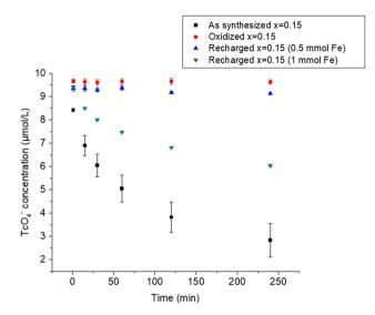
Fig. 8  $TcO_4^-$  reduction kinetics in x=0.15 nanoparticles: as-synthesized material, oxidized material, and oxidized material recharged with 0.5 and 1 mmol FeCl<sub>2</sub>.
