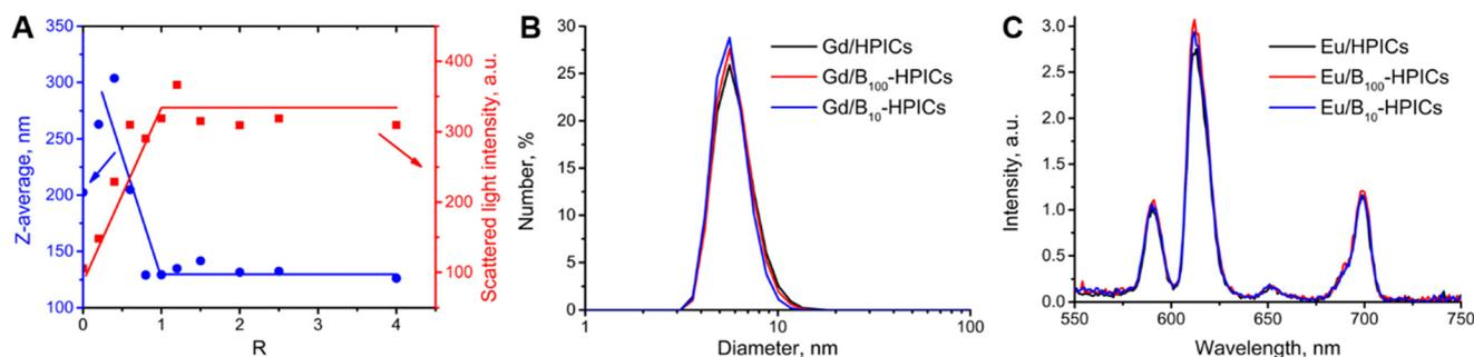
**Fig. 2** (A) Evolution of Z-Average and scattered light intensity measured by DLS for an aqueous solution of Gd/B<sub>10</sub>-HPICs as a function of ratios  $R$  ([polymer] = 0.5 wt%; lines are just guide for the eye). (B) Number-averaged hydrodynamic diameter distributions of Gd/HPICs, Gd/B<sub>100</sub>-HPICs and Gd/B<sub>10</sub>-HPICs ( $R = 1$ ). (C) Emission spectra of Eu/HPICs, Eu/B<sub>100</sub>-HPICs and Eu/B<sub>10</sub>-HPICs at  $R = 1$ .
