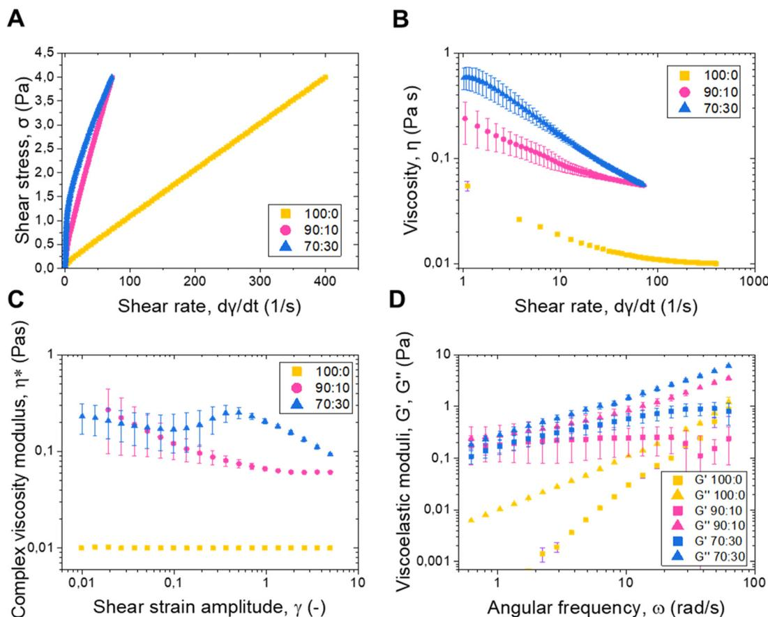
**Fig. 4** Rheological characterization of the NLS. (A) Shear stress ( $\sigma$ ) as a function of the shear rate ( $\dot{\gamma}$ ). (B) Viscosity ( $\eta$ ) as a function of the shear rate ( $\dot{\gamma}$ ). (C) Relationship between the modulus of the complex viscosity ( $\eta^*$ ) and the shear strain amplitude ( $\gamma$ ). (D) Viscoelastic moduli  $G'$  and  $G''$  as a function of the angular frequency  $\omega = 3$ .
