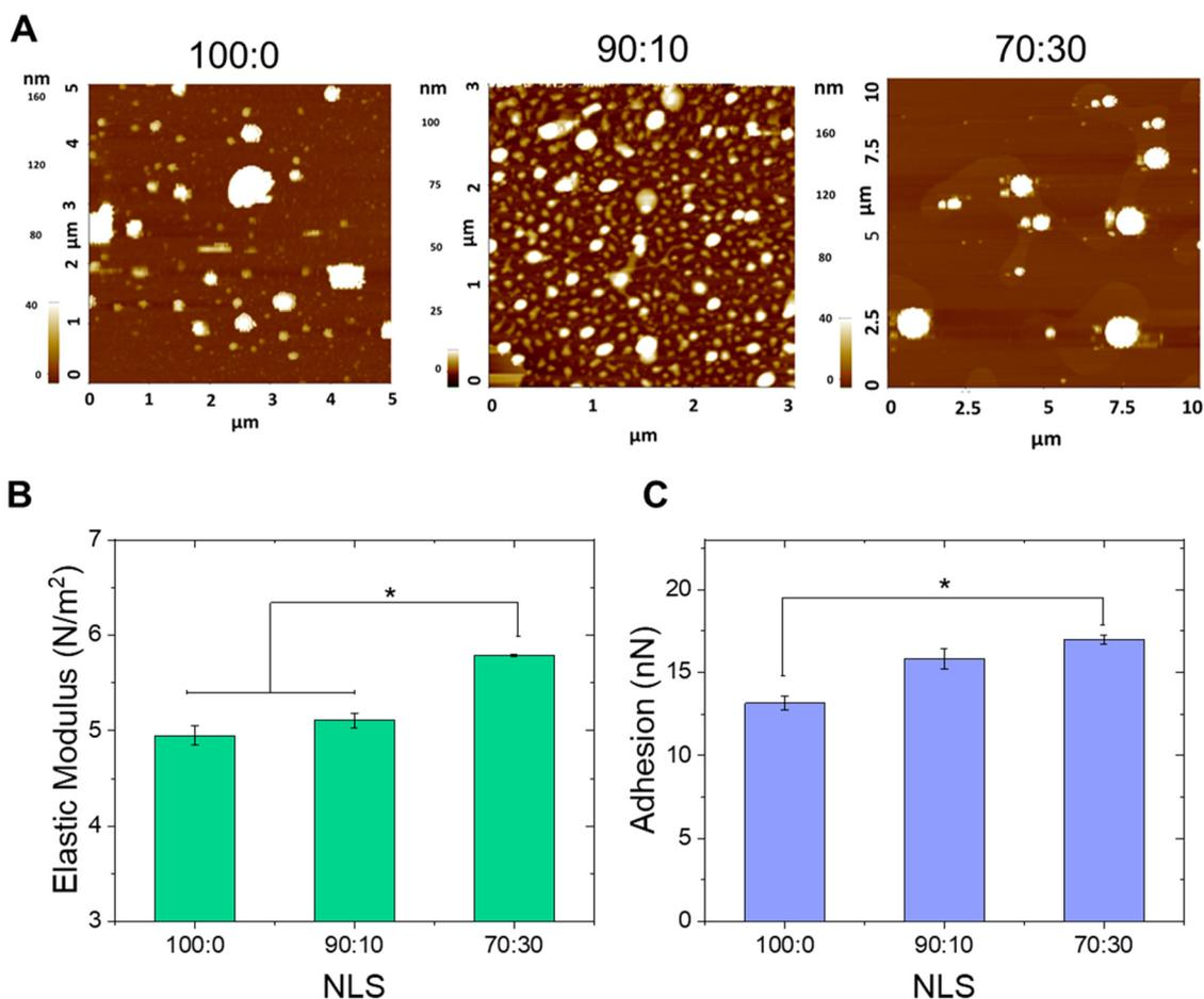
**Fig. 3** Characterization of NLS mechanical properties. (A) Topographic images of NLS (100 : 0, 90 : 10, and 70 : 30). The z-range of the AFM images is indicated on the colour bar. (B) Elastic modulus and (C) adhesion of the NLSs measured by Atomic Force Spectroscopy (AFM) in Pin-point mode. One-way ANOVA followed by Tukey's *post hoc* test showed significant differences between all groups ( $p < 0.05$ )  $n = 30$ .
