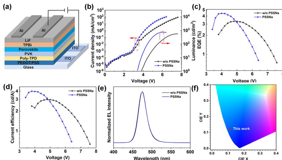
**Fig. 4** Optimization of device performance by modified PEDOT:PSS hole transport layer. (a) Device structure diagram. (b)  $J$ - $L$ - $V$  characteristics. (c) EQE versus voltage curves. (d) Current efficiency versus voltage curves. (e) EL spectra at the voltage corresponding to the maximum EQEs. (f) CIE coordinates.
