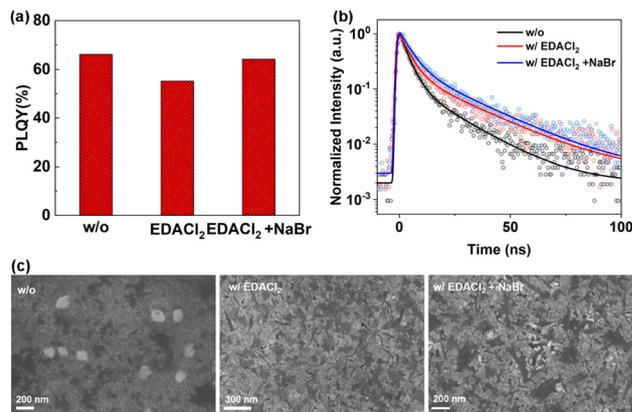
**Fig. 3** Radiation mechanism and surface morphology analysis of quasi-2D perovskite films. (a) PLQYs excited using a 365 nm LED, and (b) photoluminescence decay at the emission peaks excited with 375 nm laser pulses (68.8 ps, 1 MHz, 10 nJ cm<sup>-2</sup>) the films of w/o, w/EDACl<sub>2</sub>, and w/EDACl<sub>2</sub> + NaBr, respectively. (c) SEM images of three kinds of films.
