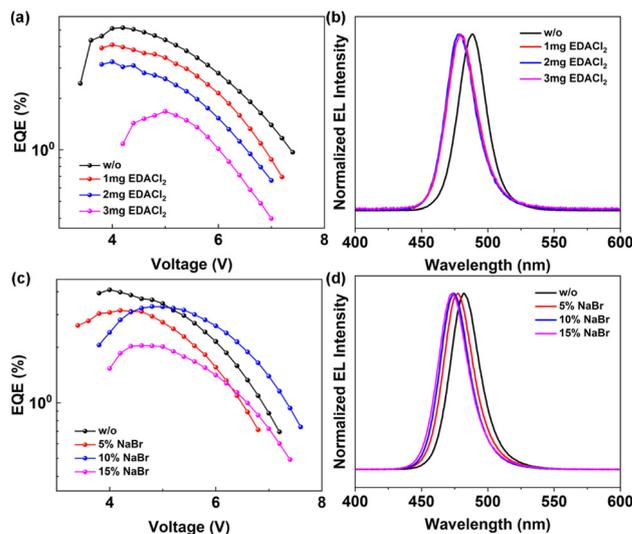
**Fig. 1** Device performance of PeLEDs with different content of EDACl<sub>2</sub> and NaBr. (a, c) EQE versus voltage curves. (b, d) EL spectra at the voltage corresponding to the maximum EQEs.
