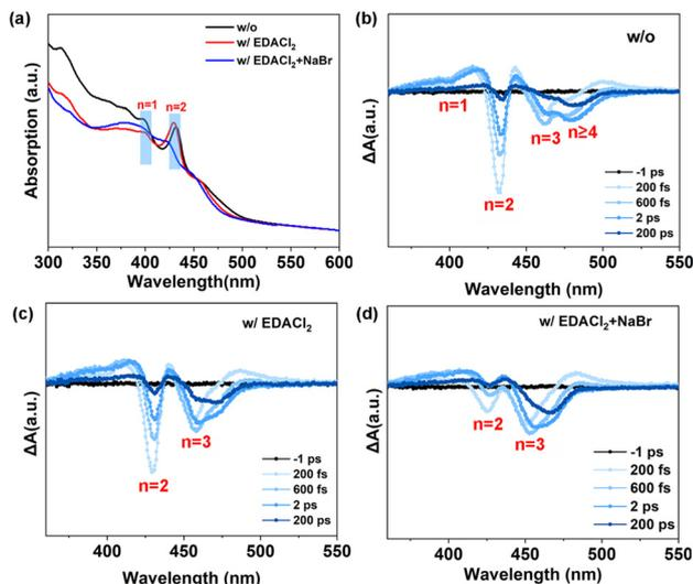
Fig. 2 Optical properties of quasi-2D perovskite films. (a) Absorption spectra and (b–d) TA spectra at different probe delay times for the films of w/o, w/EDACl<sub>2</sub>, and w/EDACl<sub>2</sub> + NaBr, respectively, following excitation at 360 nm (100 fs, 1 kHz, 1.6 μJ cm<sup>-2</sup>).
