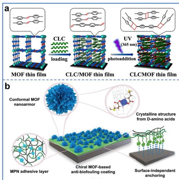
**Fig. 8** (a) Preparation of CLCMOF membrane by encapsulation of CLC into the pores of achiral MOFs. Reproduced with permission from ref. 58. Copyright 2024, American Chemical Society. (b) Preparation of chiral MOF membrane (MPN-DMOF) by reaction of chiral ligands with MPN matrix. Reproduced with permission from ref. 59. Copyright 2024, Wiley-VCH.
