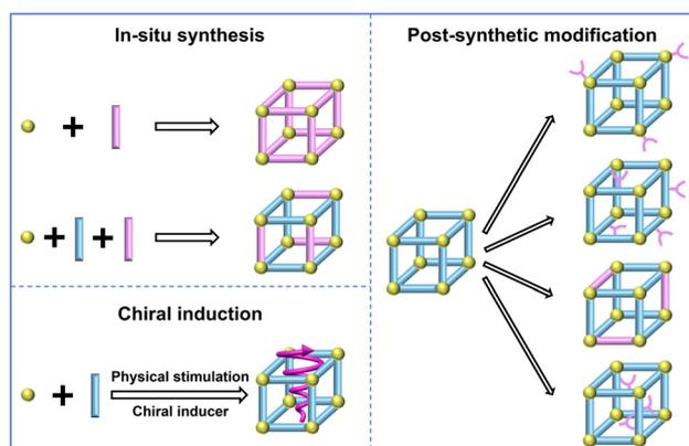
**Fig. 4** Preparation methods for chiral MOFs include *in situ* synthesis, post-synthetic modification, and chiral induction. Yellow balls represent metal nodes, blue sticks represent organic ligands, purple sticks represent chiral ligands, and purple Y-shaped curves represent chiral molecules.
