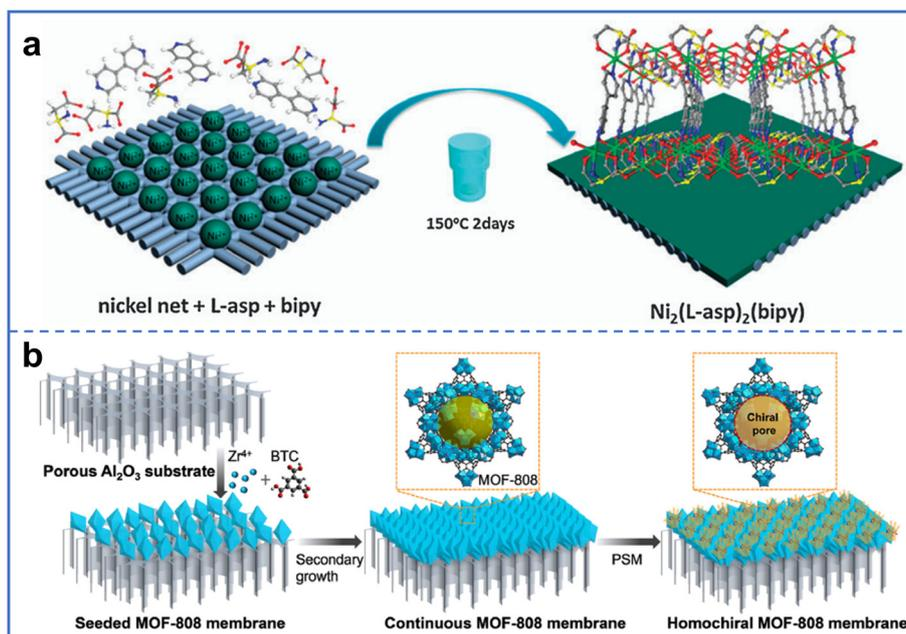
**Fig. 2** (a) Preparation of thin chiral  $\text{Ni}_2(\text{L-asp})_2(\text{bipy})$  membrane with Ni net as both substrate and metal source. Reproduced with permission from ref. 27. Copyright 2013, The Royal Society of Chemistry. (b) Preparation of chiral MOF-808 membranes by introduction of chiral molecules to MOF-808 membranes. Reproduced with permission from ref. 23. Copyright 2024, American Chemical Society.
