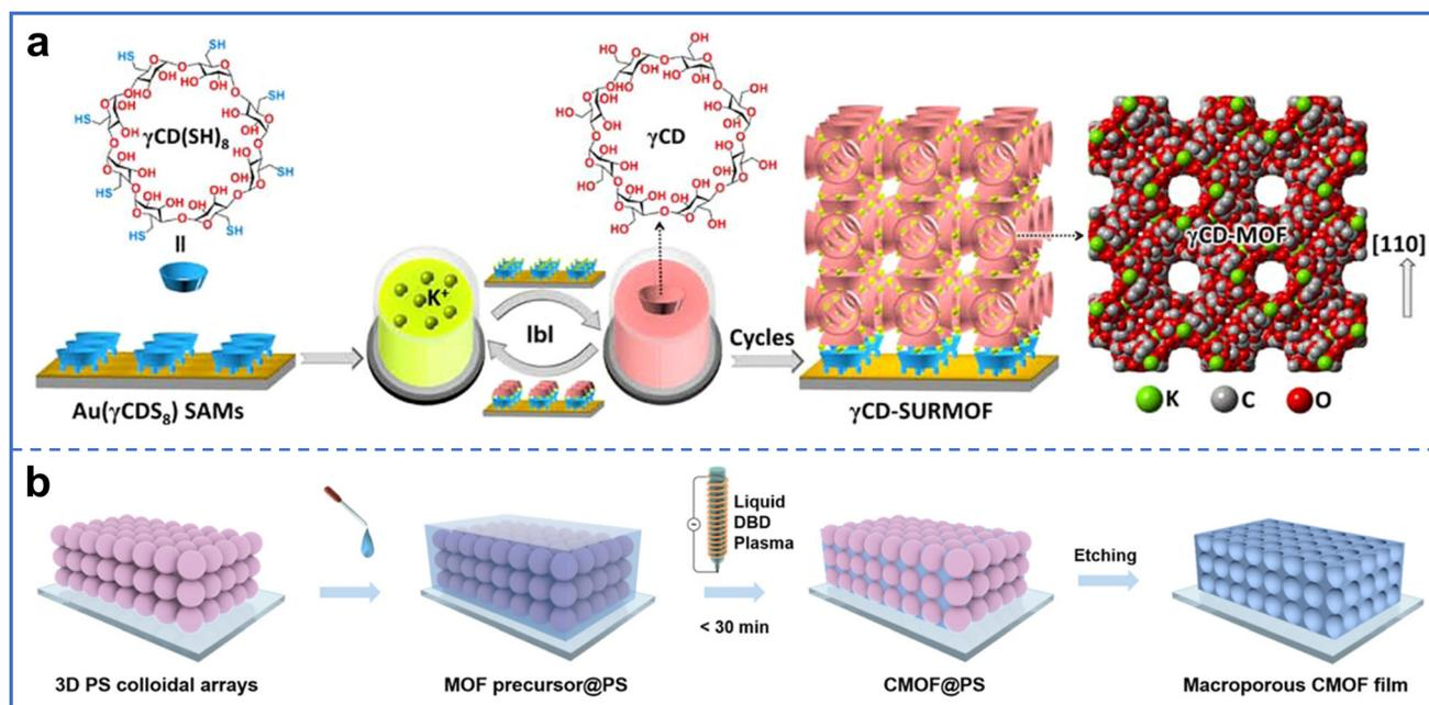
**Fig. 3** (a) Preparation of  $\gamma$ CD-SURMOF membrane by assembly of metal ions and ligands layer by layer onto  $\gamma$ CD(SH)<sub>8</sub> modified Au substrates. Reproduced with permission from ref. 29. Copyright 2022, Chinese Chemical Society. (b) Preparation of M-CMOF membranes with hierarchical porous structures by using PS arrays as templates. Reproduced with permission from ref. 30. Copyright 2024, American Chemical Society.
