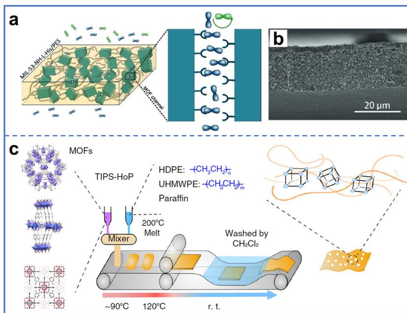
**Fig. 7** (a) Preparation of self-supporting MMMs by solution casting method with chiral MIL-53-NH-L-His dispersed in PES. (b) SEM image of the cross-section of MMMs with 20 wt% MIL-53-NH-L-His loading. Reproduced with permission from ref. 44. Copyright 2019, Wiley-VCH. (c) Preparation of MMMs with high MOF loading by chiral Zn-BLD dispersed in mixed HDPE and UHMWPE polymers through TIPS-HoP method. Reproduced with permission from ref. 55. Copyright 2019, Springer Nature.
