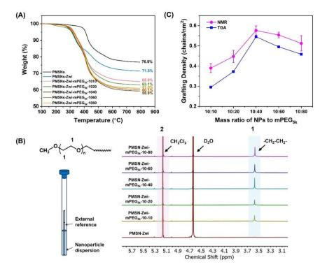
**Fig. 1** PEGylation quantification of MSN NPs analyzed by TGA and qNMR. (A) Thermal curves from TGA of PMSN, PMSN-Zwi, and PMSN-ZwimPEG<sub>5k</sub> NPs with different mPEG<sub>5k</sub> amounts. (B) Schematic illustration of the quantification of PEG chains by <sup>1</sup>H NMR spectroscopy. (C) Comparison of grafting densities obtained from TGA and qNMR.
