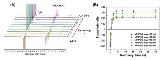
Fig. 2 (A) The original NMR spectra of the spin-lattice relaxation time ( $T_1$ ) delay experiment. The recovery time ( $\tau$ ) varied from 10 ms to 30 s, with intensities measured at 13 incremental recovery times. (B) T1 analysis and fitted curves with one-phase exponential decay function with time constant parameter ( $y = B + F \times \exp(-\tau/T_1)$ , eqn (3)).
