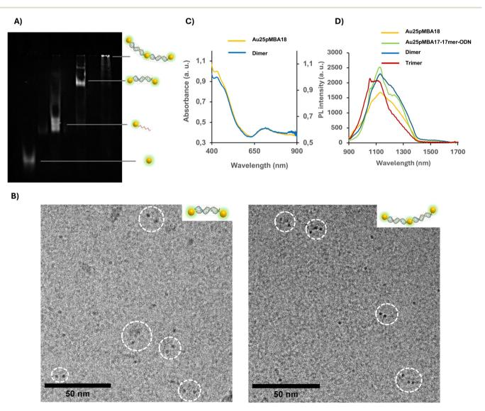
Fig. 5 (A) Native PAGE analysis of the hybridization reaction resulting in the Au<sub>25</sub>(pMBA)-17mer dimer and trimer structures, image was taken using an NIR-II camera; the original gel is shown in Fig. S11.† (B) Absorbance and (C) PL spectra of dimers in comparison with free AuNCs dispersed in water;  $\lambda_{exc.}$  808 nm. (D) TEM images of the Au<sub>25</sub>(pMBA)-17mer dimer and trimer structures.
