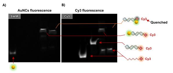
Fig. 4 Native PAGE analysis of the coupling between Cy3 dye and AuNCs through DNA hybridization (17-mer). Gel imaging was recorded using an NIR-II camera (A) and a BioRad gel imager with a Cy3 filter (B). The original gel is shown in Fig. S8.†
