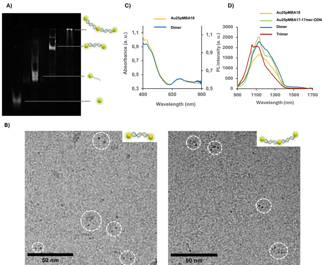
Fig. 5 (A) Native PAGE analysis of the hybridization reaction resulting in the Au<sub>25</sub>(pMBA)-17mer dimer and trimer structures, image was taken using an NIR-II camera; the original gel is shown in Fig. S11.† (B) Absorbance and (C) PL spectra of dimers in comparison with free AuNCs dispersed in water;  $\lambda_{\text{exc}}$ . 808 nm. (D) TEM images of the Au<sub>25</sub>(pMBA)-17mer dimer and trimer structures.
