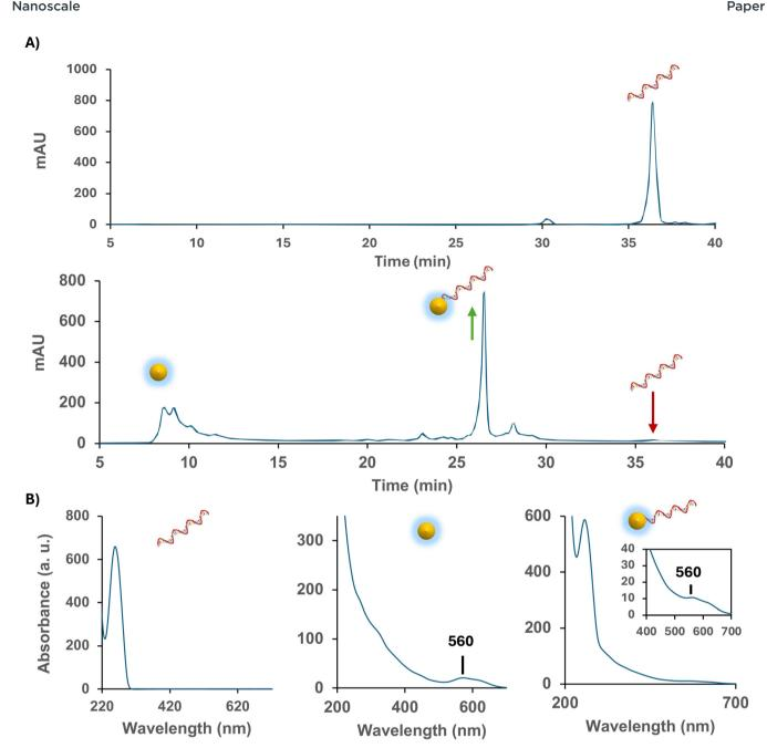
Fig. 3 (A) Top shows the RP-HPLC analysis for thiol-17mer, while the bottom shows the RP-HPLC analysis for Au<sub>18</sub>(SG)<sub>14</sub> conjugated with thiol-17mer with a linear gradient from 0% to 12% of acetonitrile in 10 mM TEAA, and detection at 260 nm. (B) Corresponding absorbance measurements of the three peaks assigned to thiol-17mer, Au<sub>18</sub>(SG)<sub>14</sub>, and Au<sub>18</sub>(SG)<sub>13</sub>-17mer<sub>(1)</sub>.
