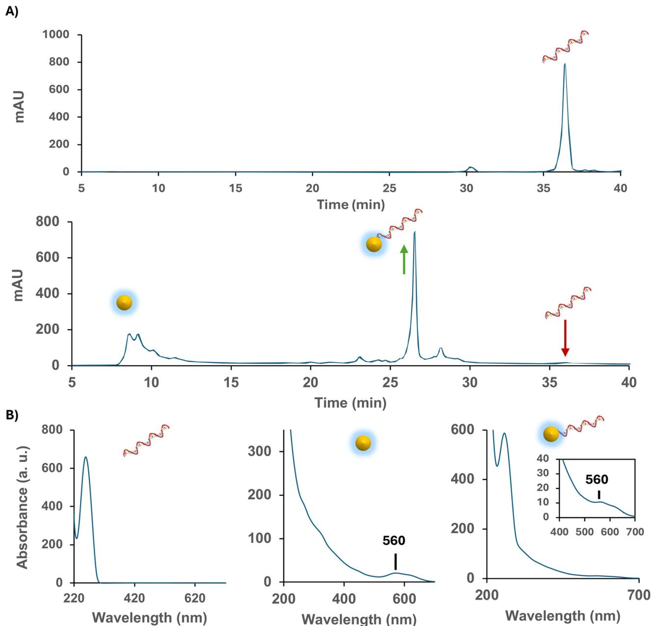
**Fig. 3** (A) Top shows the RP-HPLC analysis for thiol-17mer, while the bottom shows the RP-HPLC analysis for  $\text{Au}_{18}(\text{SG})_{14}$  conjugated with thiol-17mer with a linear gradient from 0% to 12% of acetonitrile in 10 mM TEAA, and detection at 260 nm. (B) Corresponding absorbance measurements of the three peaks assigned to thiol-17mer,  $\text{Au}_{18}(\text{SG})_{14}$ , and  $\text{Au}_{18}(\text{SG})_{13}$ -17mer<sub>(1)</sub>.
