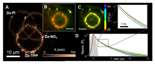
Fig. 4 Photografting chemically complex structures, composed of Dz-TPP (bottom), fluoresceine modified alkyne layer (left), and *p*-nitro-benzene diazonium (right). (A) AFM characterization of the layers thickness (B) RGB image of the fluorescence emission, (C) FLIM characterization of the layer, along with its associated (D) photoluminesence decay curves, where the incident pulse width is also shown (gray).
