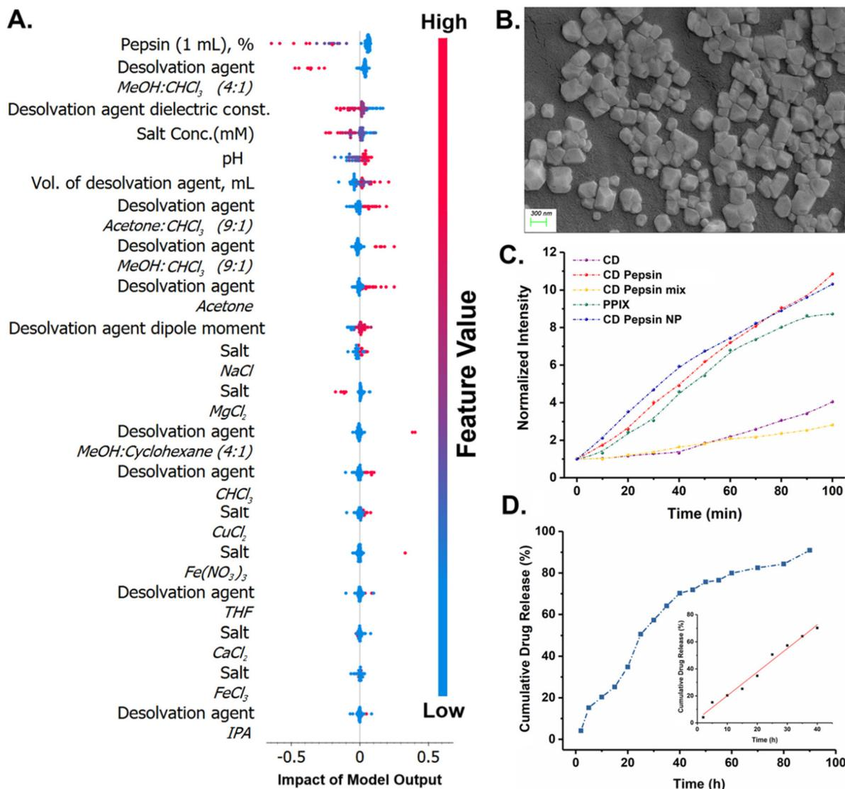
**Fig. 4** (A) SHAP summary plot for the neural network model for class 1 of CD-pepsin NPs, (B) FE-SEM image of Dox loaded CD-pepsin NPs, (C) Comparison of ROS generation efficiency of CDs, CD-pepsin, the CD-pepsin physical mixture, PpIX, and CD-pepsin NPs and (D) *in vitro* drug release profile of DOX from CD-pepsin NPs; inset: Linearity over the range 0–40 h.
