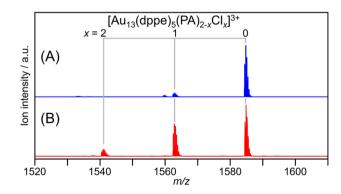
Fig. 1 Positive-ion ESI mass spectra of (A) 20:(Cl<sup>-</sup>)3 and (B) the product obtained by mixing 20·(Cl<sup>-</sup>)<sub>3</sub> and [BF<sub>4</sub>]<sup>-</sup> in acetonitrile solution.
