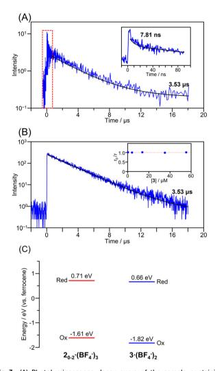
Fig. 3 (A) Photoluminescence decay curve of the sample containing the  $2_0$  monomer and the  $(2_1)_2$ Fe dimer. The inset shows an enlarged decay curve around 0-80 ns. (B) Photoluminescence decay curve of the building block cluster  $2_{0-2}$ . The inset shows the Stern-Volmer plot based on the luminescence lifetimes of  $2_{0-2}$  in the presence of 3 as a quencher. (C) Redox potentials of  $2_{0-2} \cdot (BF_4^-)_3$  and  $3 \cdot (BF_4^-)_2$ .
