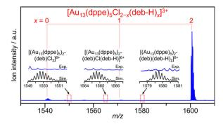
Fig. 4 Positive-ion ESI mass spectrum of the product obtained by mixing 1 and deb- $H_2$  in acetonitrile solution in the presence of a base.
