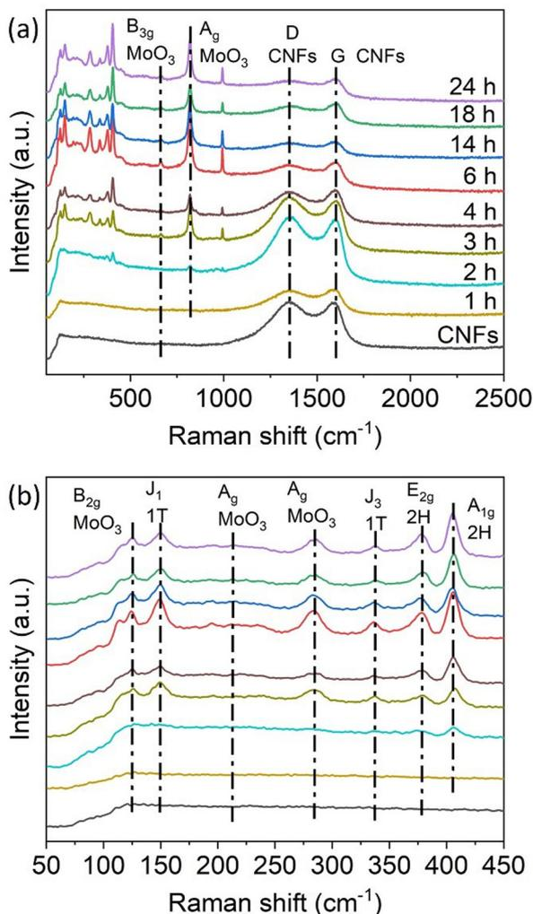
Fig. 3 (a) Raman spectra of the 1T-MoS<sub>2</sub>/CNFs hybrids labelled with the reaction time. (b) Magnification of the Raman spectra of the hybrids in the range of 50–450 cm<sup>-1</sup>.
