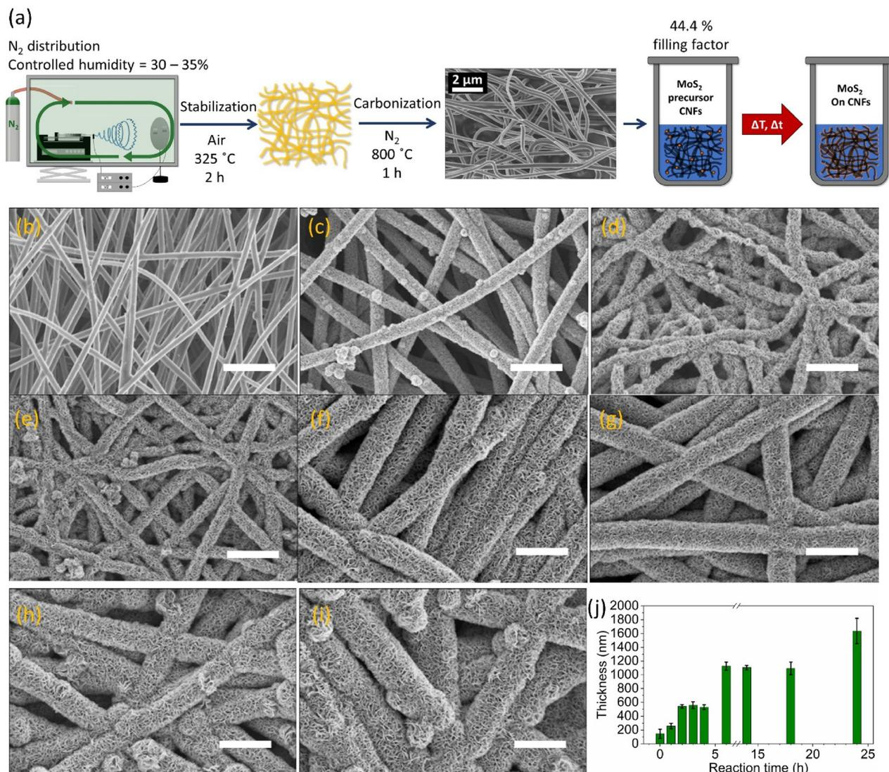
**Fig. 1** (a) Schematic representation of the 1T-MoS<sub>2</sub>/CNFs nanohybrids production process and SEM image of pristine CNFs from the three-steps process. SEM of 1T-MoS<sub>2</sub>/CNFs samples with the reaction time of (b) 1 h, (c) 2 h, (d) 3 h, (e) 4 h, (f) 6 h, (g) 14 h, (h) 18 h, and (i) 24 h. Scale bar: 2  $\mu$ m. (j) Relationship between the diameter of the hybrid samples and the reaction time.
