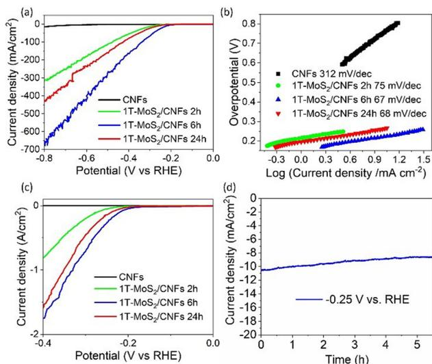
**Fig. 7** (a) LSV, (b) Tafel slope and (c) ECSA-normalized polarization curves of pristine CNFs and of the 1T-MoS<sub>2</sub>/CNFs hybrids. (d) Chronoamperometry plot of 1T-MoS<sub>2</sub>/CNFs 6 h, plotted at a constant volt of  $-2.5$  V vs. RHE.
