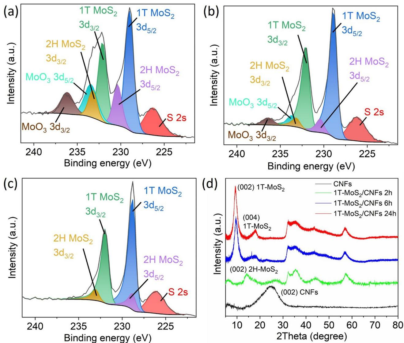
Fig. 4 Mo 3d high-resolution XPS spectra of (a) 1T-MoS<sub>2</sub>/CNFs 2 h, (b) 1T-MoS<sub>2</sub>/CNFs 6 h and (c) 1T-MoS<sub>2</sub>/CNFs 24 h. (d) XRD patterns of CNFs and the representative 1T-MoS<sub>2</sub>/CNFs hybrids.
