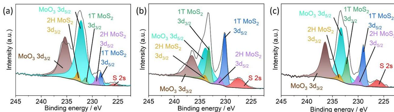
Fig. 6 Mo 3d high-resolution XPS spectra of (a) 1T-MoS<sub>2</sub>/CNFs 2 h, (b) 1T-MoS<sub>2</sub>/CNFs 6 h and (c) 1T-MoS<sub>2</sub>/CNFs 24 h after the GCD test.
