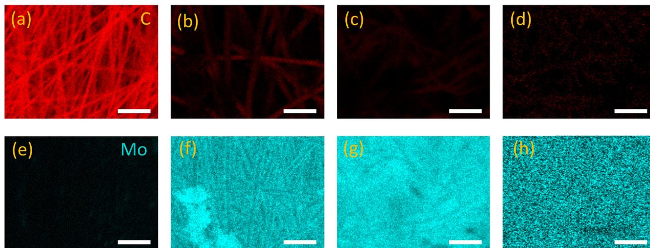
Fig. 2 EDX mapping of C and Mo in the 1T-MoS<sub>2</sub>/CNFs hybrids. C mapping of 1T-MoS<sub>2</sub>/CNFs with the reaction time of (a) 1 h, (b) 2 h, (c) 3 h and (d) 4 h. Mo mapping of 1T-MoS<sub>2</sub>/CNFs with the reaction time of (e) 1 h, (f) 2 h, (g) 3 h and (h) 4 h. Scale bar: 2.5  $\mu$ m.
