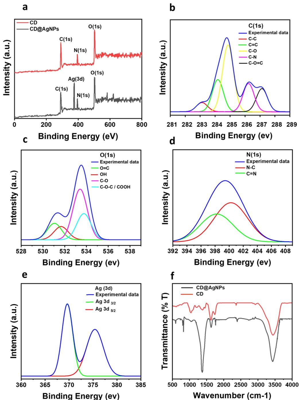
**Fig. 3** Analysis of the structural characteristics of CDs and the CD@AgNP hybrid prepared by the green synthesis method. (a) Full XPS spectrum of CDs and the CD@AgNP hybrid, (b) C 1s photoelectron spectrum, (c) XPS spectrum of the N 1s peak, (d) O 1s XPS spectrum, (e) XPS spectrum of the Ag 3d peak, and (f) FTIR spectra of the synthesized CDs and CD@AgNPs.
