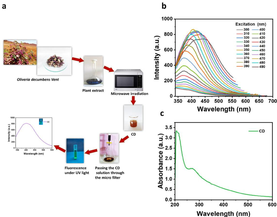
**Fig. 1** (a) Schematic illustration of the green synthesis of carbon dots from *Oliveria decumbens Vent.* extract as a precursor, (b) excitation wavelength-dependent fluorescence spectra and (c) the absorption spectrum of the as-synthesized carbon dots.
