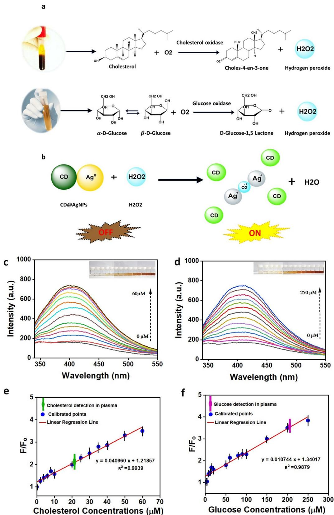
**Fig. 6** (a) Schematic detection of cholesterol and glucose based on the enzymatic reaction-assisted approach and (b) etching of AgNPs in the CD@AgNP hybrid. Changes in the fluorescence spectrum as a function of (c) cholesterol (2–60  $\mu\text{M}$ ) and (d) glucose (4–250  $\mu\text{M}$ ) concentration and the corresponding calibration curves for (e) cholesterol and (f) glucose. The conditions are the same for all samples.
