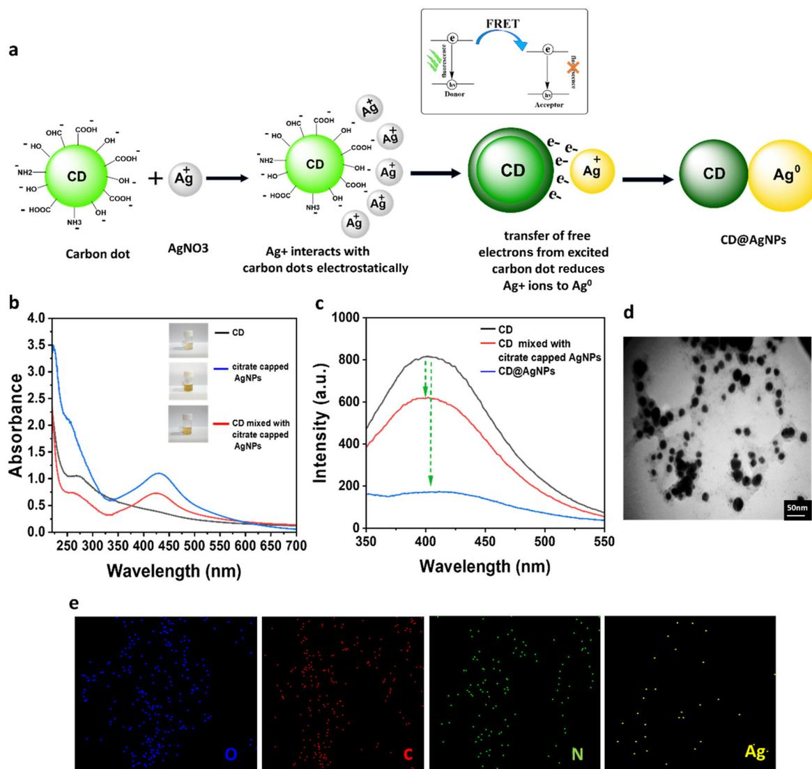
**Fig. 2** (a) Schematic illustration of the formation of the CD@AgNP hybrid. (b) UV-visible spectrum of CDs, AgNPs with citrate coating, a mixture of CDs with citrate-coated AgNPs, and the CD@AgNP hybrid. (c) Fluorescence emission spectrum of CDs, the mixture of CDs with citrate-coated AgNPs and the CD@AgNP hybrid. (d) TEM images of CD@AgNPs. (e) EDX image of the dispersion of each of the elements constituting CD@AgNPs: O element, C element, N element, and Ag element.
