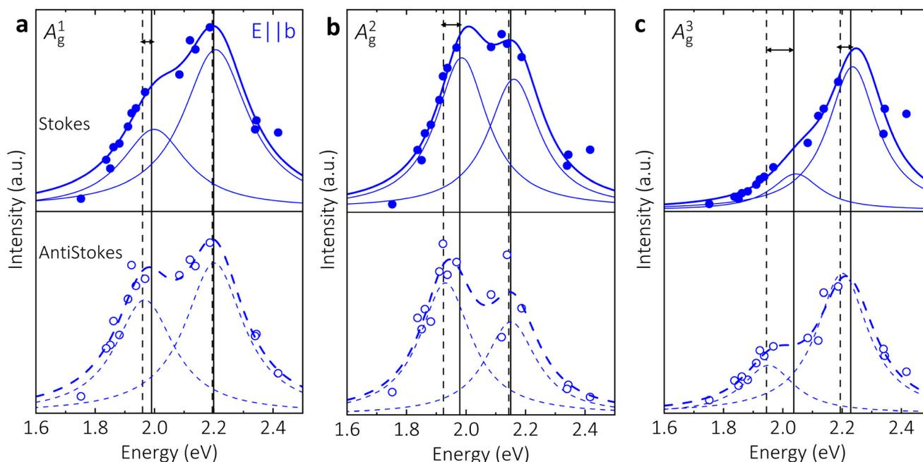
**Fig. 2** Resonant Raman excitation profile: Resonant Raman profiles of the (a)  $A_g^1$ , (b)  $A_g^2$ , and (c)  $A_g^3$  modes for both Stokes (solid circles and curves) and anti-Stokes (empty circles and dashed curves) regions for laser co-polarized along b-axis. The symbols denote the experimental data points, while the solid and dashed blue curves are the fits using eqn (1).
