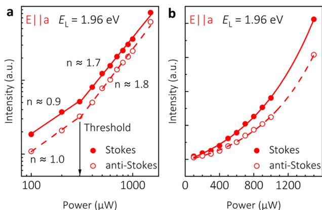
**Fig. 4** Stimulated Raman scattering: Integrated Stokes and anti-Stokes  $A_{g2}^2$  intensities vs. laser power under  $E_L = 1.96 \text{ eV}$  excitation in (a) log–log and (b) linear–linear scales, respectively. Symbols denote the data points, while the solid and dashed lines are the linear (a) and exponential (b) fits, respectively. The laser power threshold for the SRS process was 300  $\mu\text{W}$ .
