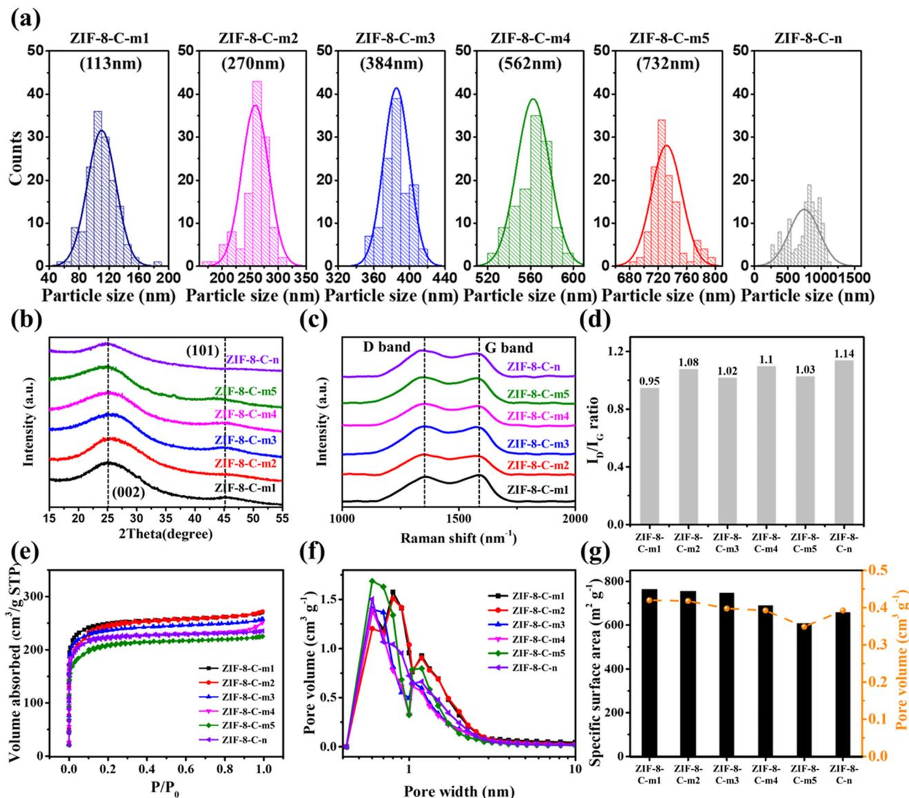
Fig. 3 (a) Particle size distribution, (b) XRD patterns, (c) Raman spectra, (d) intensity ratio of the D-band to the G-band ( $I_D/I_G$  ratio), (e)  $N_2$  adsorption–desorption isotherms, (f) pore size distribution, and (g) Brunauer–Emmett–Teller (BET) surface area and pore volume of ZIF-8-C samples.
