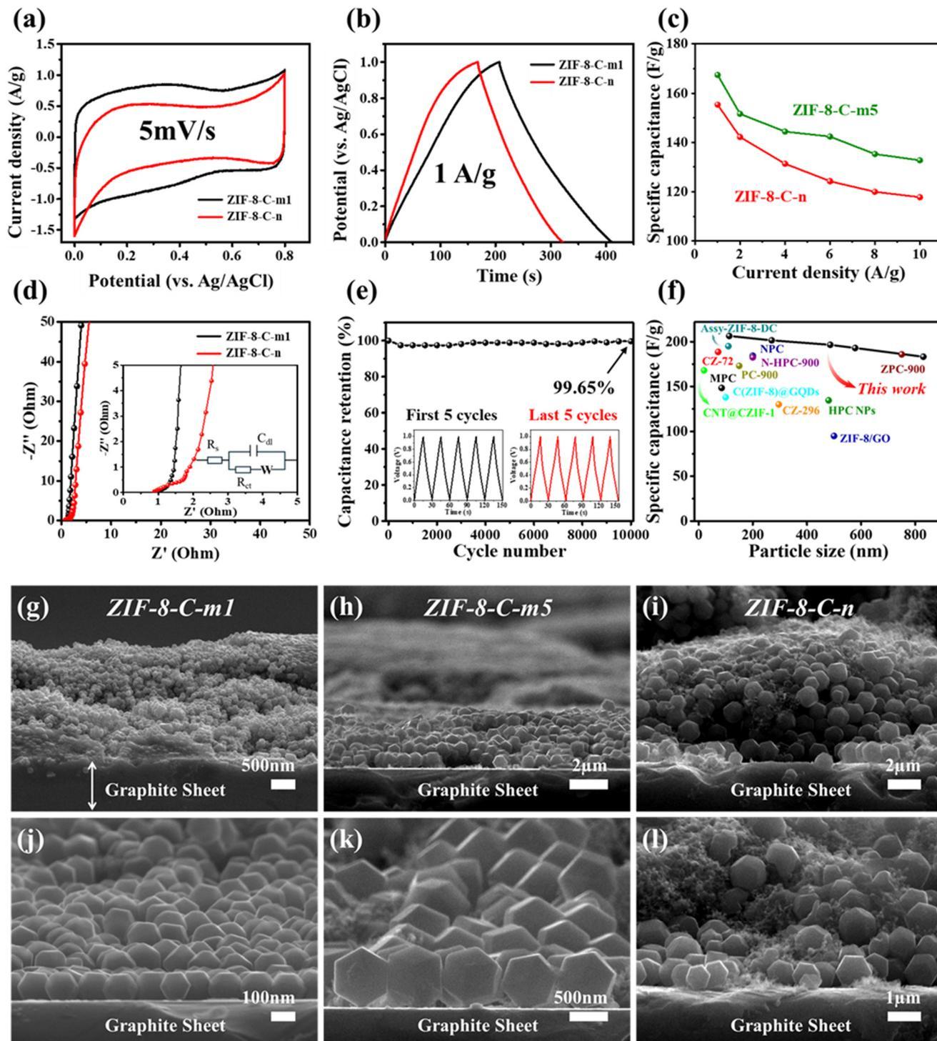
**Fig. 6** (a) CV curves, (b) GCD curves, (c) capacitance retention at different current densities, and (d) Nyquist plots of ZIF-8-C-m1, ZIF-8-C-m5, and ZIF-8-C-n (inset: Randles equivalent circuit); (e) cycling stability of ZIF-8-C-m1 at  $10 \text{ A g}^{-1}$  across 10 000 cycles; and (f) relative capacitance of ZIF-8-derived carbon samples of varying sizes. Low- and high-magnification SEM cross-sectional images of (g and j) ZIF-8-C-m1, (h and k) ZIF-8-C-m5, and (i and l) ZIF-8-C-n.
