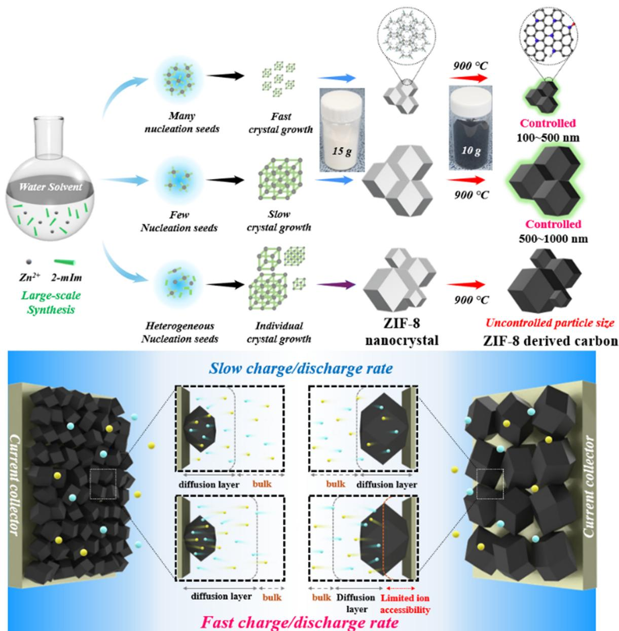
**Fig. 1** Schematic of the preparation methods for ZIF-8-C with various particle sizes and size distributions, and the effect of particle size on the supercapacitor performance.
