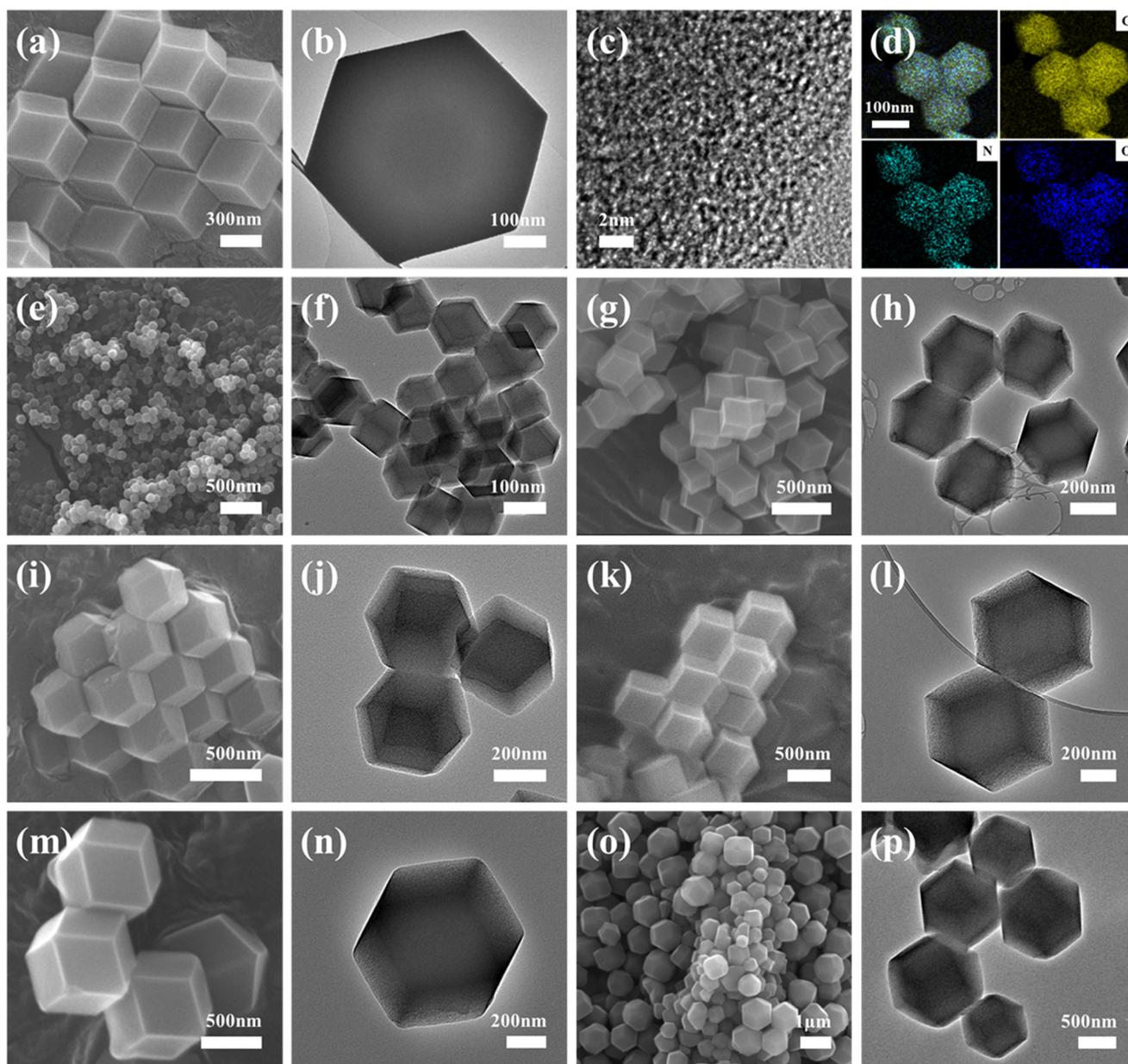
**Fig. 2** (a) Scanning electron microscopy (SEM) and (b) transmission electron microscopy (TEM) images of ZIF-8 nanocrystals. (c) High-magnification TEM image and (d) TEM-energy dispersive X-ray spectroscopy (EDS) mapping of ZIF-8-C-m1. SEM and TEM images of (e and f) ZIF-8-C-m1, (g and h) ZIF-8-C-m2, (i and j) ZIF-8-C-m3, (k and l) ZIF-8-C-m4, (m and n) ZIF-8-C-m5, and (o and p) ZIF-8-C-n.
