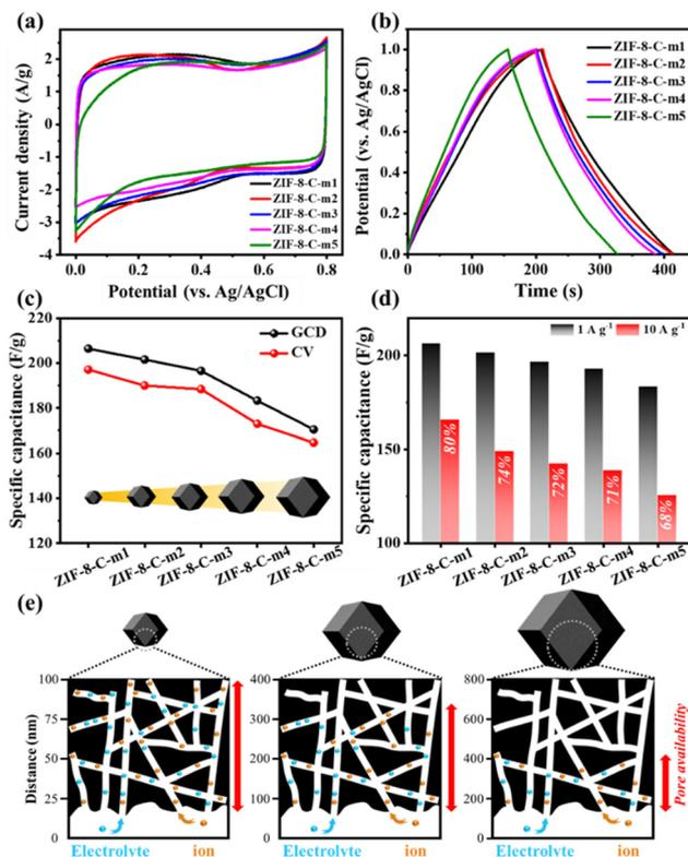
**Fig. 5** (a) CV curves (10 mV s<sup>-1</sup>) and (b) GCD curves (1 A g<sup>-1</sup>) of the uniform ZIF-8-C samples with different particle sizes. (c) Relative specific capacitance of the uniform ZIF-8-C samples with different particle sizes and (d) at different current densities. (e) Schematic representation of electrolyte ion accessibility differences according to particle size.
