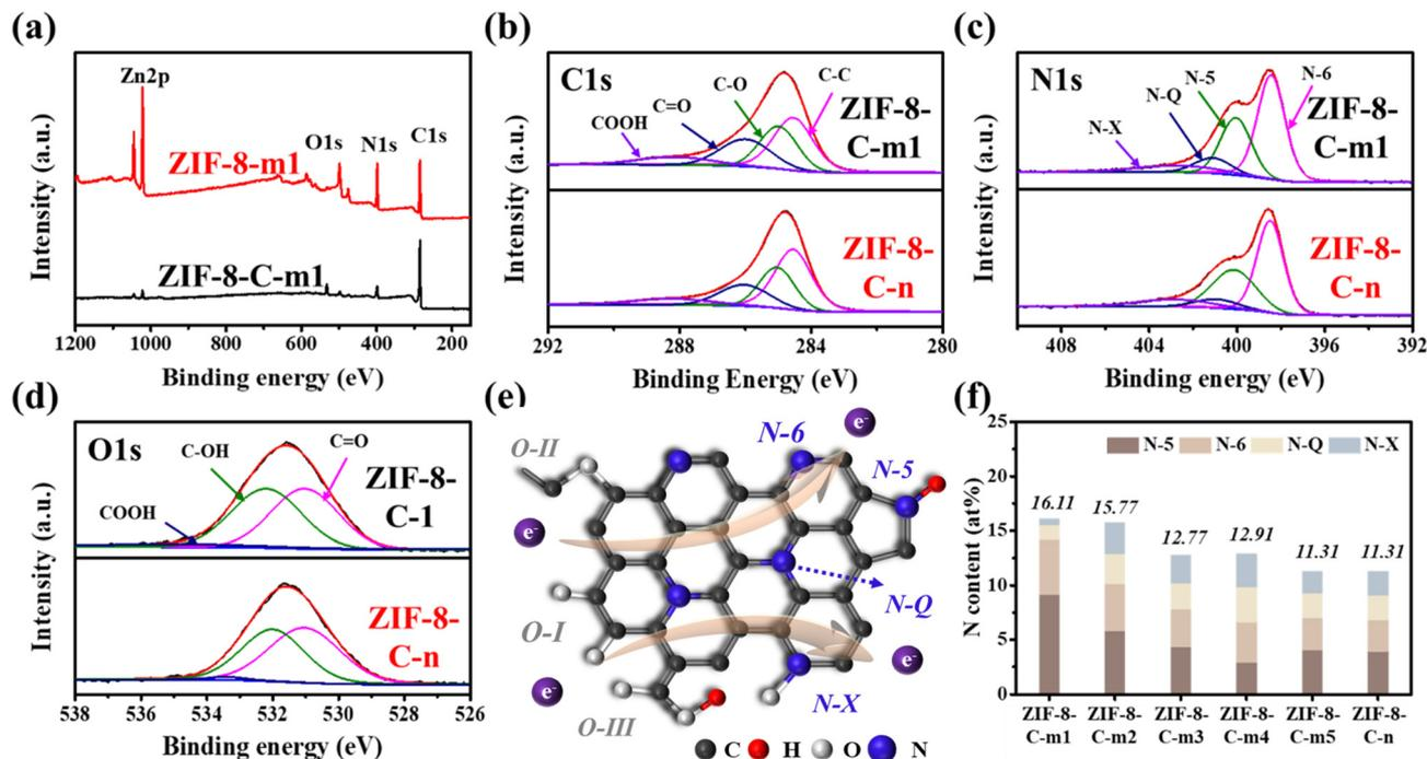
Fig. 4 (a) XPS profiles of ZIF-8-m1 and ZIF-8-C-m1; (b) C 1s, (c) N 1s, and (d) O 1s XPS profiles of ZIF-8-C-m1 and ZIF-8-C-n; (e) schematic model of the oxygen and nitrogen groups on the carbon samples; and (f) nitrogen atom content in all carbon samples.
