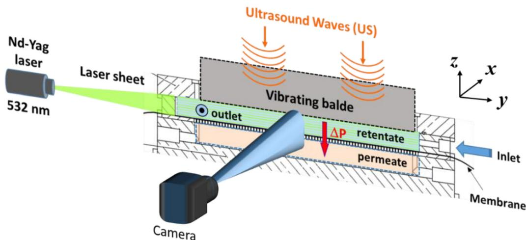
Fig. 1 In situ micro-PIV measurements under FU-US (schematic).
