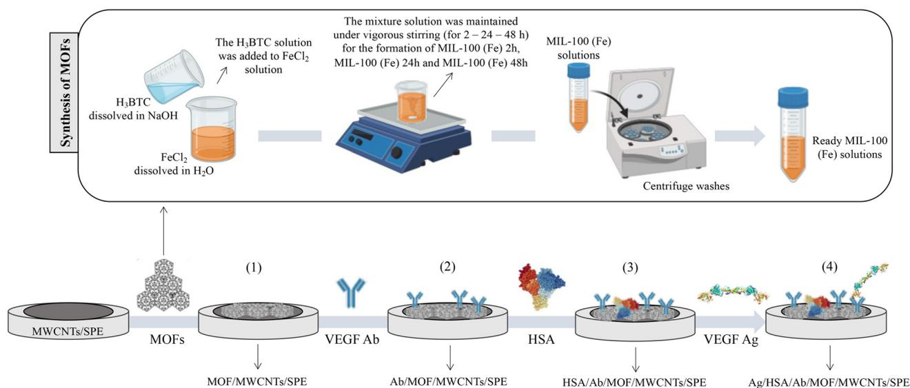
**Fig. 12** Preparation of the modified MWCNTs/SPE by (1) MOF-MIL 100(Fe) deposition, (2) VEGF Ab immobilization, (3) HSA surface blocking and (4) VEGF Ag binding. Inset: procedures for the synthesis of MIL 100(Fe) 2 h, MIL 100(Fe) 24 h and MIL 100(Fe) 48 h.
