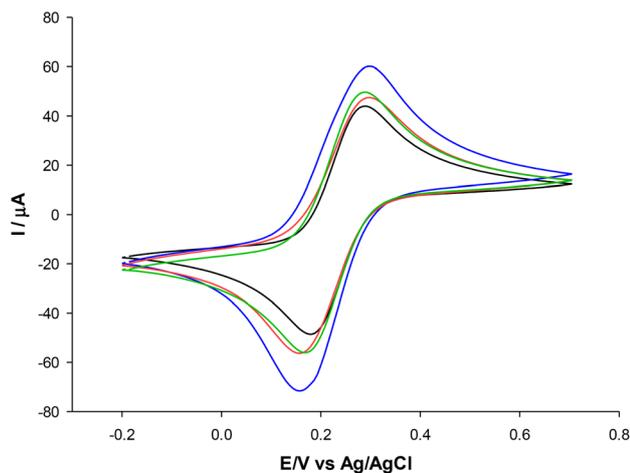
**Fig. 8** CV curves of the MWCNTs/SPE (black curve), the MIL100(Fe) 2 h/MWCNTs/SPE (red curve), the MIL100(Fe) 24 h/MWCNTs/SPE (green curve) and the MIL100(Fe) 48 h/MWCNTs/SPE (blue curve) measured in 2.5 mM Zobell's solution. Scan rate: 25 mV s<sup>-1</sup>.
