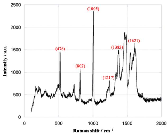
**Fig. 2** Raman spectrum of 48 h MIL-100(Fe).
