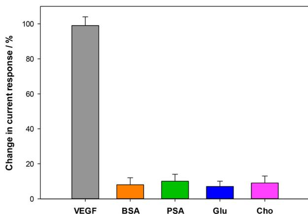
**Fig. 11** Histograms of selectivity assay for VEGF (500 pg mL<sup>-1</sup>) vs. different potential interferents (5000 pg mL<sup>-1</sup>) in 2.5 mM Zobell's solution.
