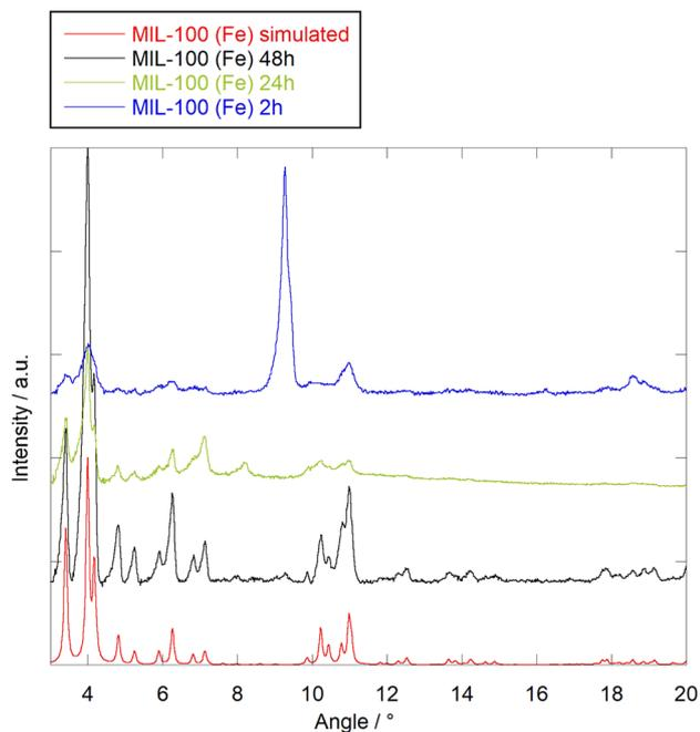
**Fig. 1** PXRD patterns of MIL-100(Fe) at 2 h (blue curve), 24 h (green curve), and 48 h (black curve) of synthesis. The red curve is the simulated spectrum of MIL-100(Fe) that is generated from the single-crystal X-ray diffraction cif file (ref. 38).
