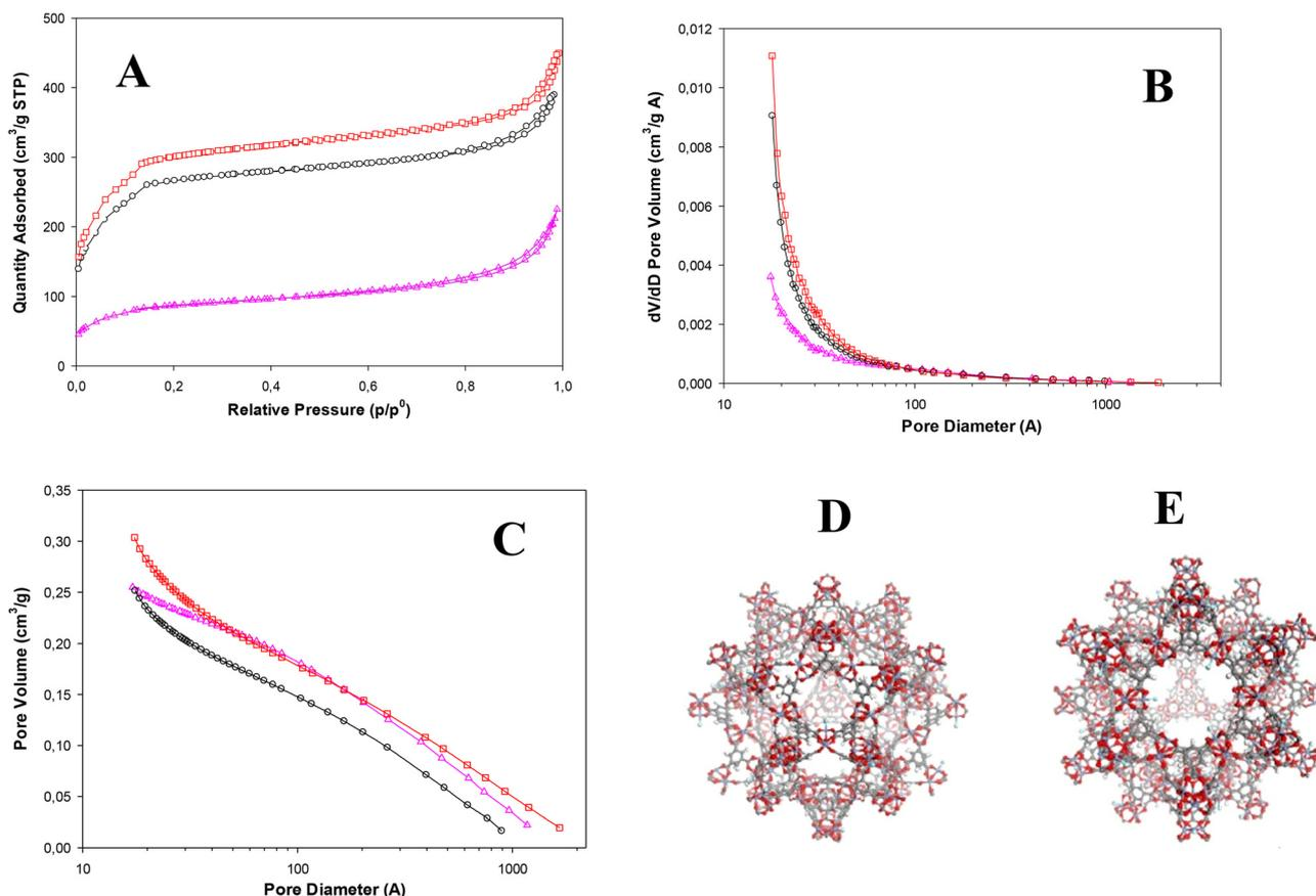
**Fig. 7** (A) BET nitrogen adsorption-desorption isotherms, (B) BJH adsorption cumulative pore volumes, and (C) BJH adsorption  $dV/dD$  pore volumes of MIL-100(Fe) at 48 h (red curve), 24 h (black curve) and 2 h (pink curve) of synthesis. MIL(100)-Fe mesoporous cages: (D) medium cage (24 Å) and (E) large cage (29 Å) (ref. 38).
