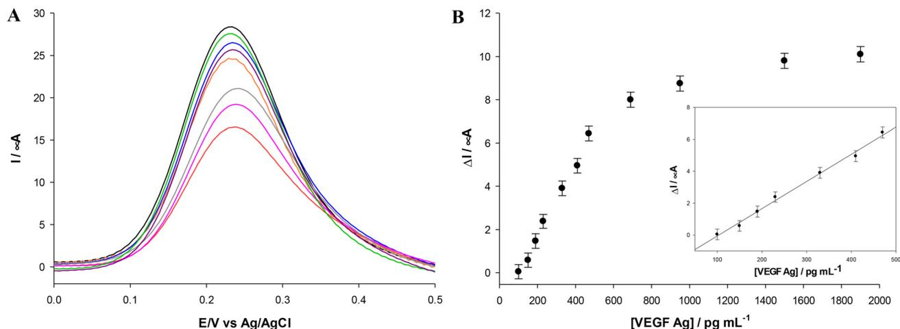
**Fig. 10** Panel A: DPV curves of the HSA/Ab/MOF/MWCNTs/SPE (black curve) modified with varying concentrations of VEGF Ag (from 150–1900  $\text{pg mL}^{-1}$ ; from green to red curves) measured in 2.5 mM Zobell's solution. Panel B: calibration plots for different VEGF concentrations (from 150–1900  $\text{pg mL}^{-1}$  in PBS pH 7.2). Inset: magnification of the linear range. Experimental conditions: 2.5 mM Zobell's solution; VEGF antibody = 10  $\text{mg mL}^{-1}$ .
