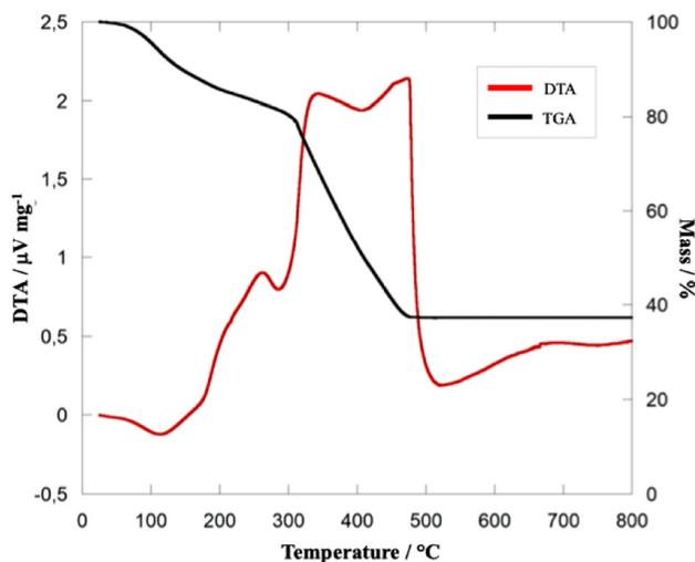
**Fig. 4** TG/DTA curves of 48 h MIL-100(Fe).
