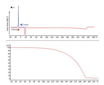
Fig. 1 DSC curve (top) and TG record (bottom) of TMT<sub>3</sub>P.
