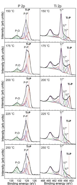
Fig. 3 High-resolution XPS spectra of P 2p and Ti 2p obtained from Ti<sub>x</sub>P<sub>y</sub> thin films after 500 ALD cycles at different deposition temperatures.
