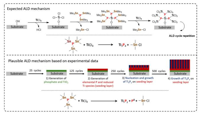
Scheme 2 (Top) Illustrative description of the expected ALD mechanism for the growth of  $Ti_x P_y$ . (Bottom) Plausible ALD mechanism proposed to describe the growth of  $Ti_x P_y$  based on experimental data.
